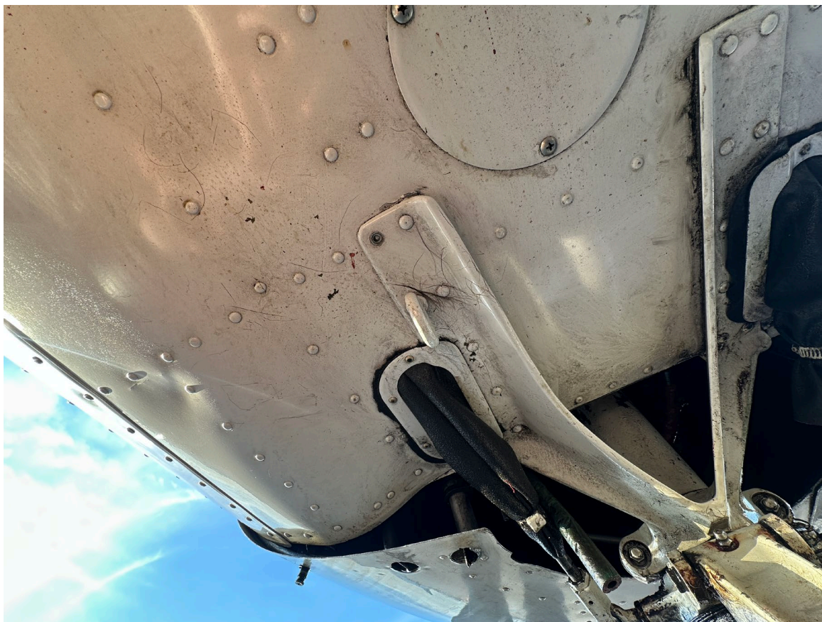
Photograph 1 - Skin deformation noted to lower left fuselage (Courtesy of FAA)
