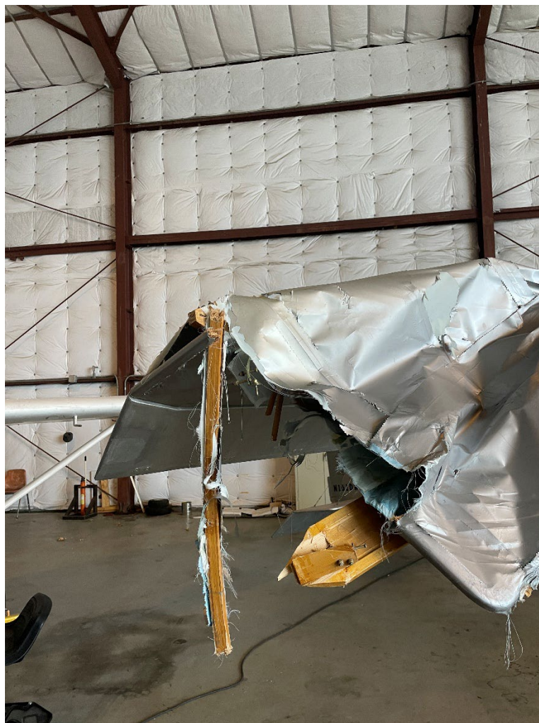
Photograph 3 - Right wing accident damage (Courtesy of FAA)
