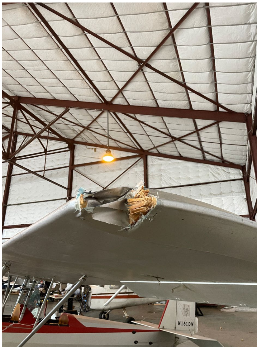
Photograph 4 - Left wing accident damage (Courtesy of FAA)
