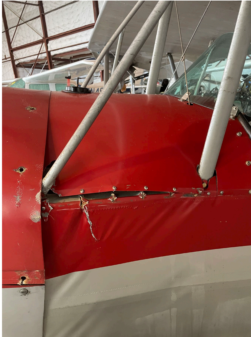
Photograph 2 - Forward left fuselage accident damage (Courtesy of FAA)
