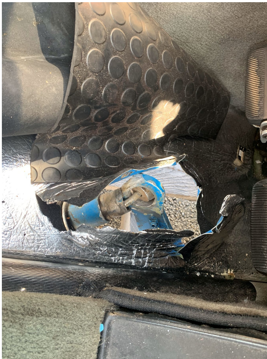
Photograph 5 - Damage to cabin floor (Source: SkyBlue Aviation)
