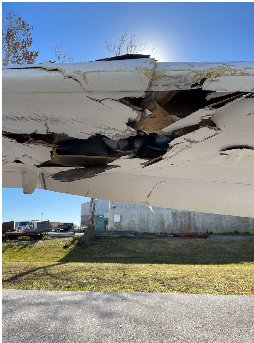
Photograph 3 - Accident Damage, Lower Forward Right Wing (Courtesy of PEA)
