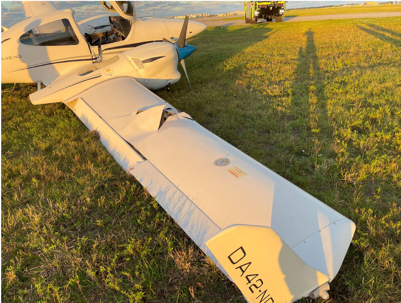
Photograph 1 - Accident Damage Right Wing (Courtesy of PEA)
