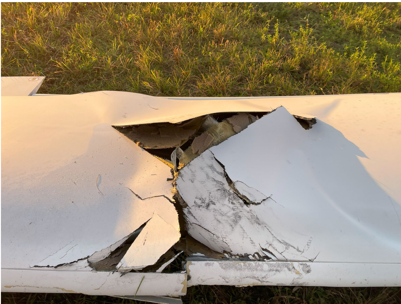
Photograph 2 - Accident Damage Upper Forward Right Wing (Courtesy of PEA)
