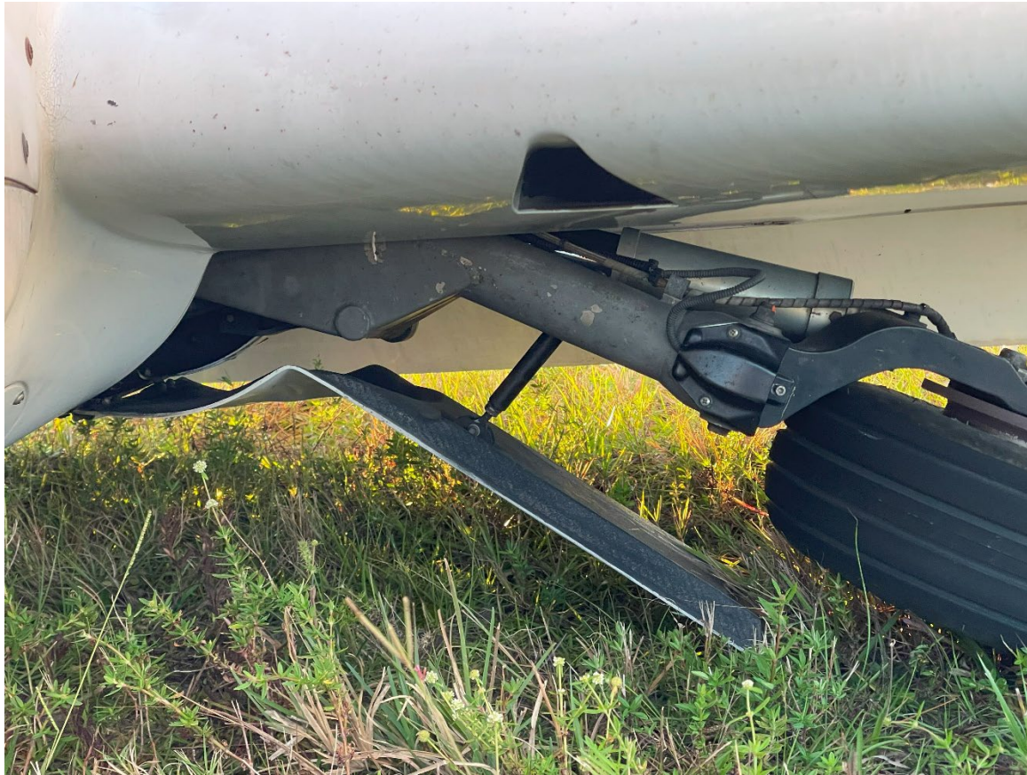
Photograph 5 - Collapsed Right Main Gear Leg (Courtesy of PEA)
