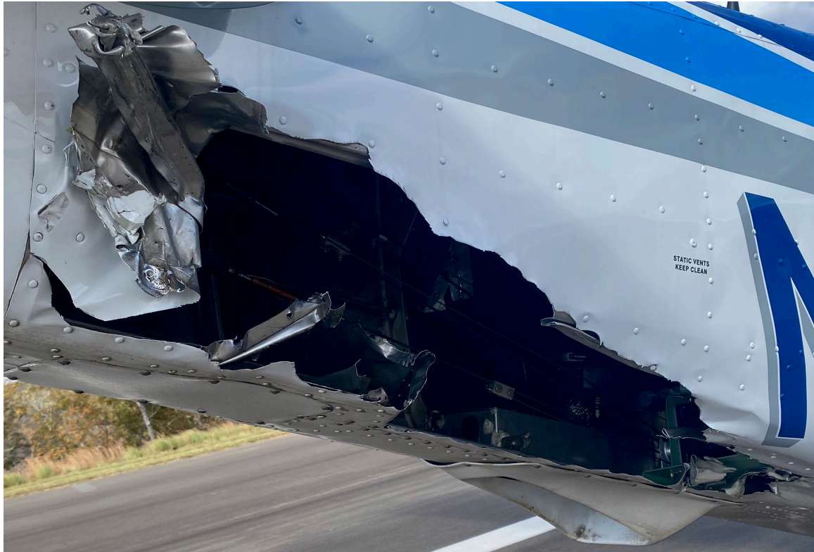
Photograph 3 - Right side tail accident damage (Courtesy of airplane owner)
