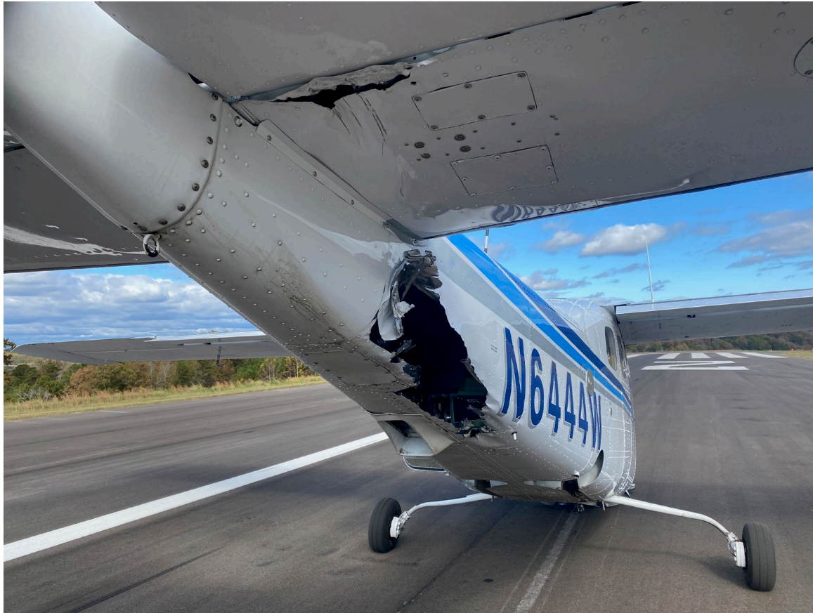
Photograph 2 - Right side tail and horizontal stabilizer accident damage (Courtesy of airplane owner)
