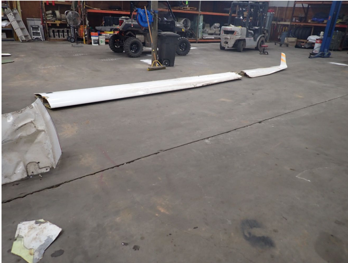
Photograph 3 - Fractured left wing (NTSB)
