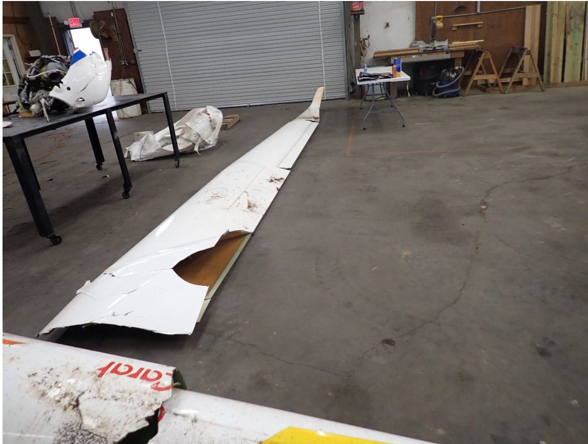
Photograph 4 - Fractured right wing (NTSB)
