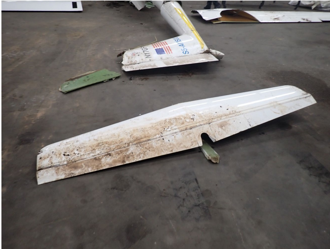
Photograph 5 - Impact separated horizontal stabilizer (NTSB)
