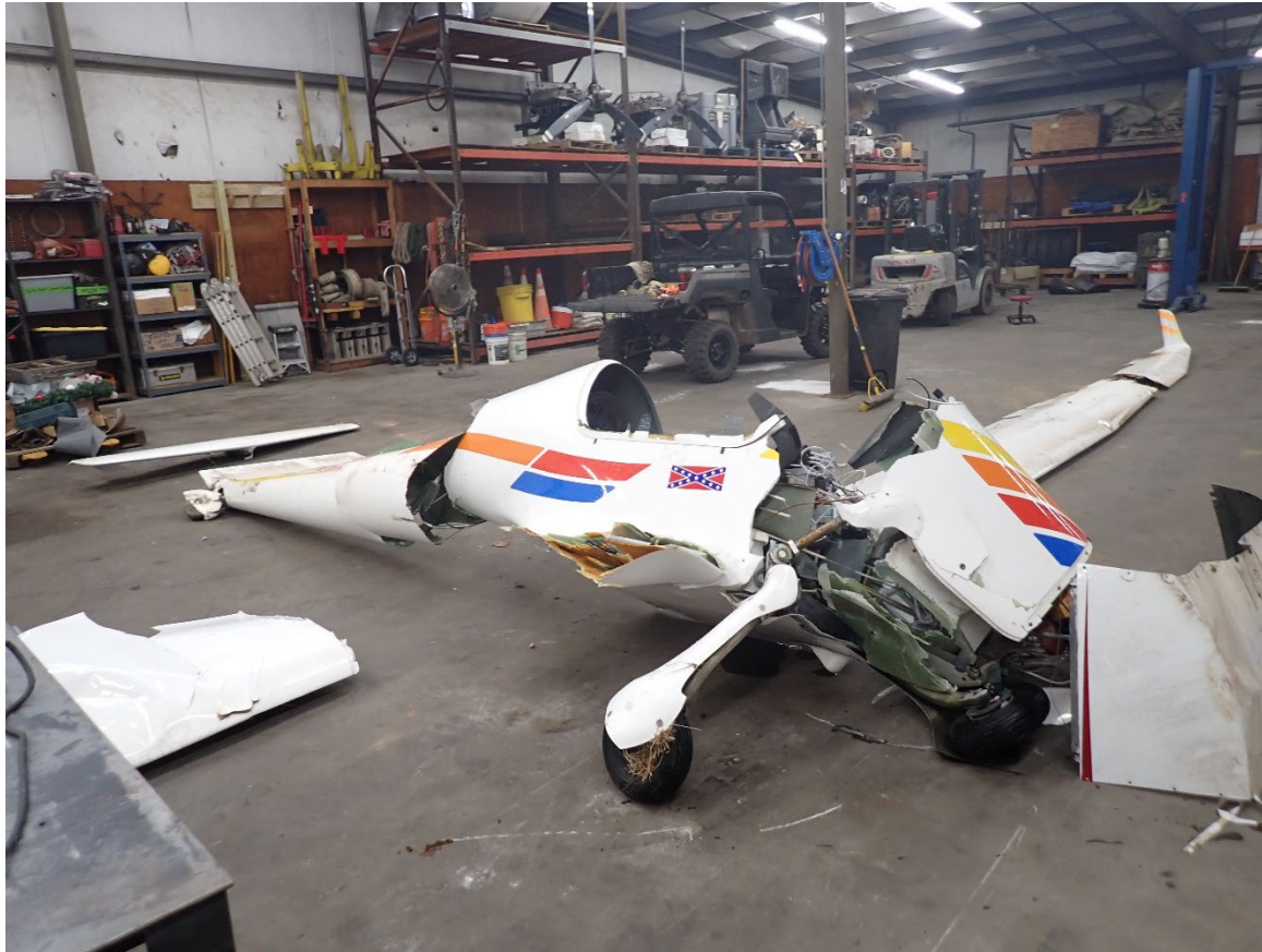
Photograph 2 - Fractured airframe (NTSB)
