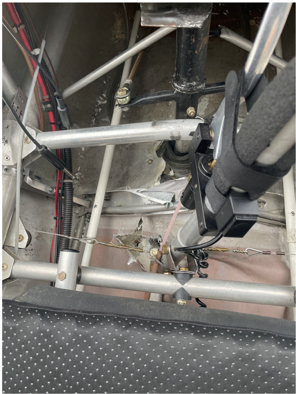
Photo 2 – View of Damage to Cabin Floor and Structure (FAA)
