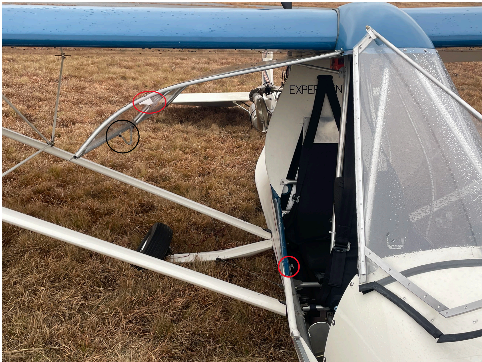
Photo 3 – View of Cabin “Gullwing” and Cockpit Doors (FAA)
