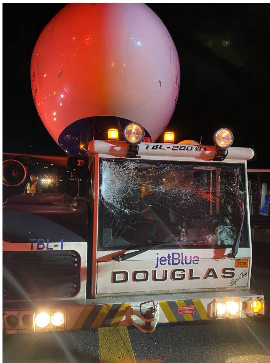
Photograph 3 - Damage noted to tug's windshield (Courtesy of FAA)
