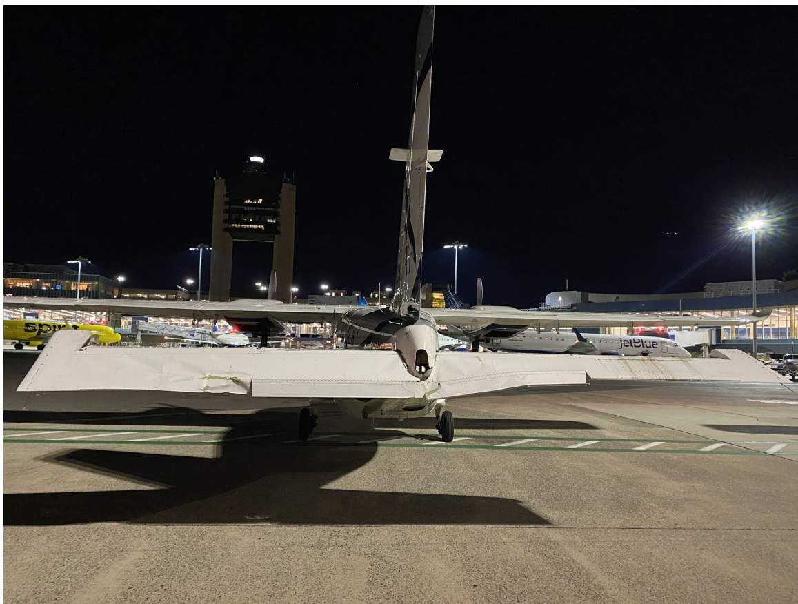
Photograph 2 - Skin deformation noted to elevator (Courtesy of FAA)
