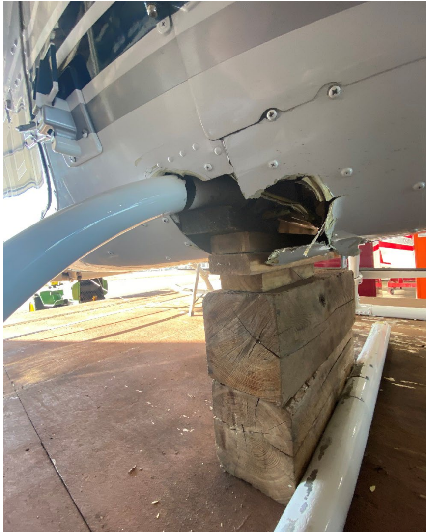
Photograph 2 - Close-up rear view of helicopter hull damage (Courtesy of FAA)
