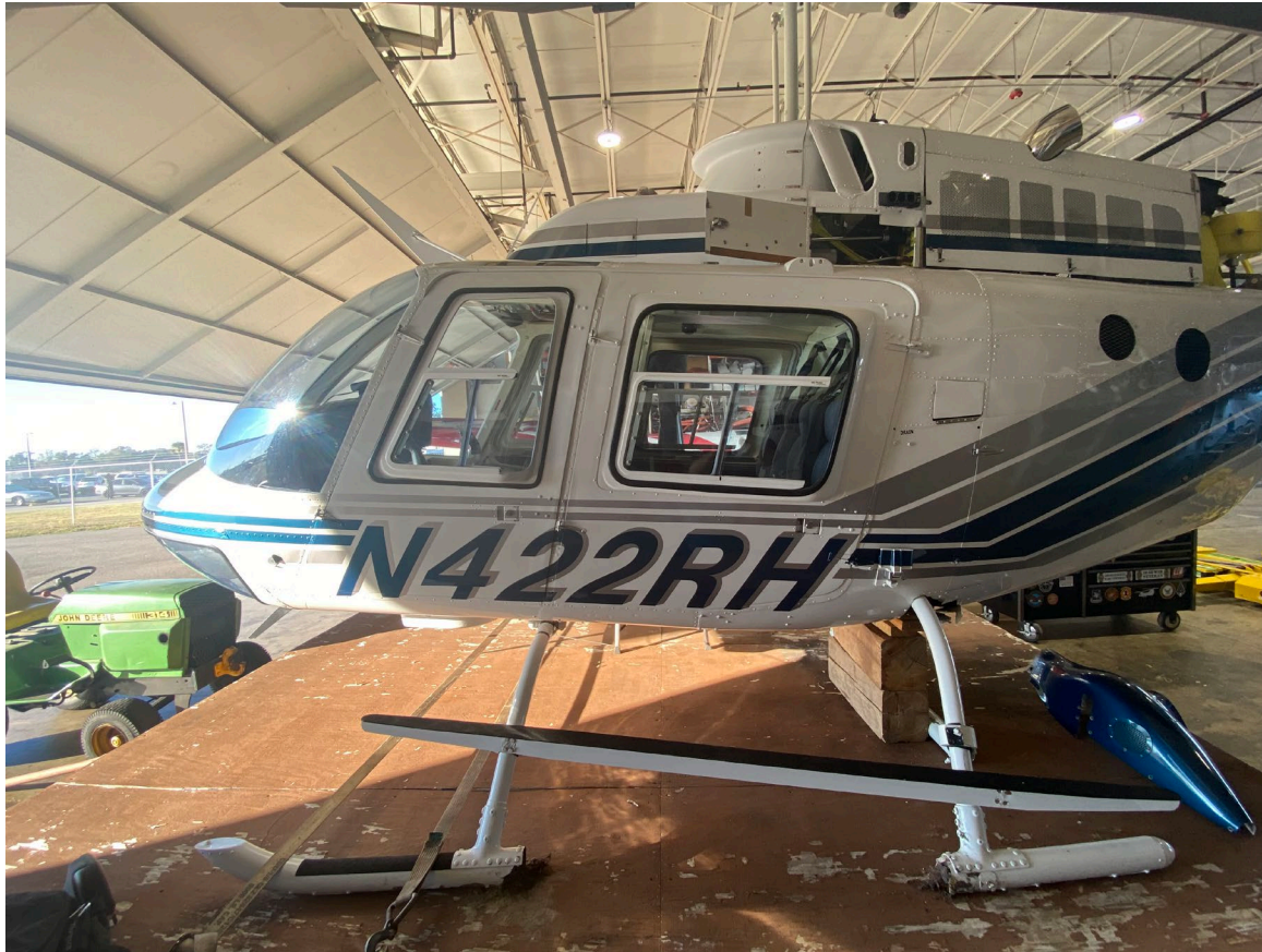
Photograph 3 - Left side view of helicopter showing landing skid damage (Courtesy of FAA)
