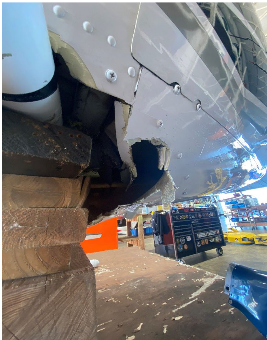
Photograph 1 - Close-up view of helicopter hull showing skid damage (Courtesy of FAA)
