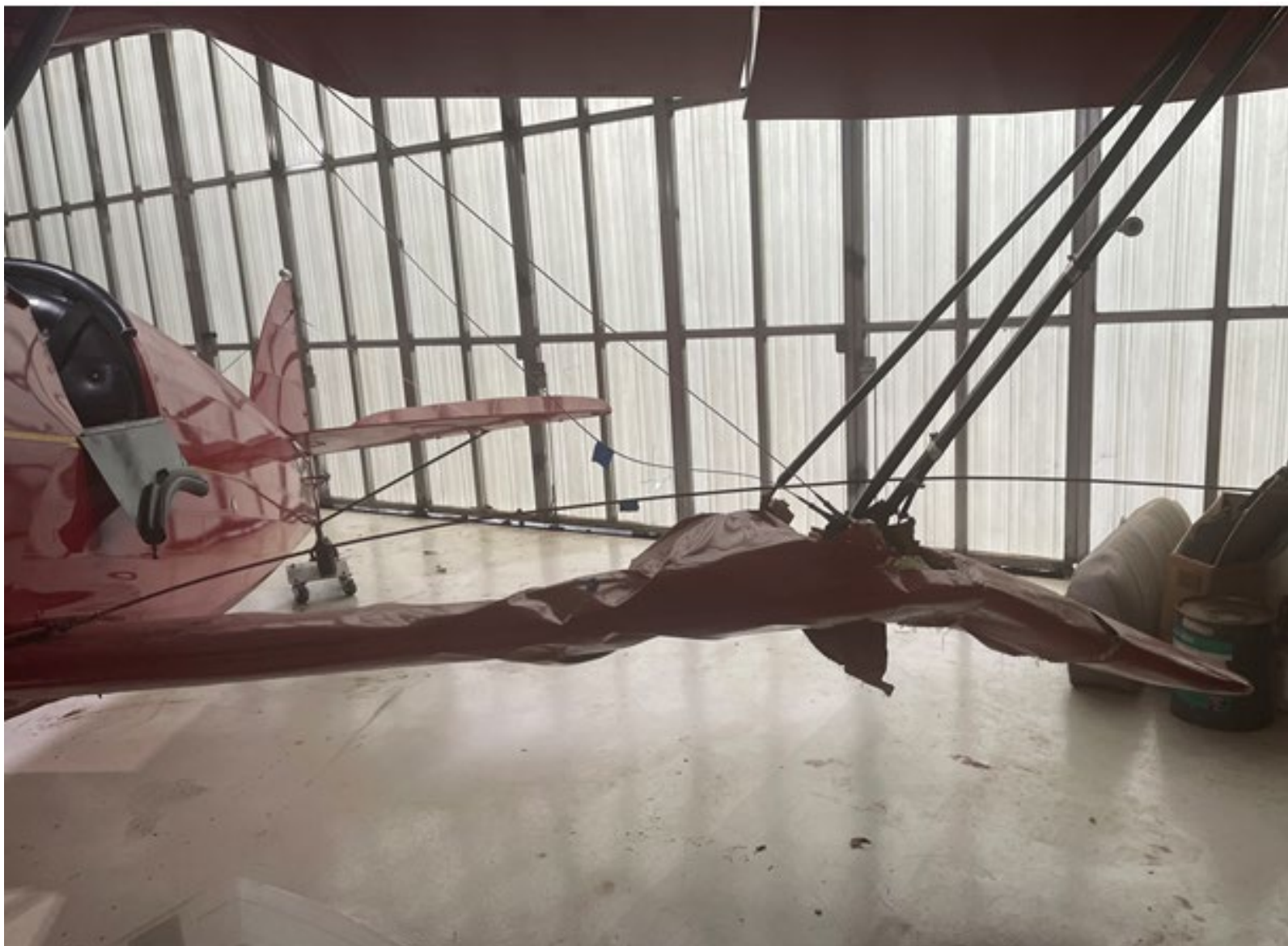
Photograph 1 - Left lower wing damage (Courtesy of FAA)
