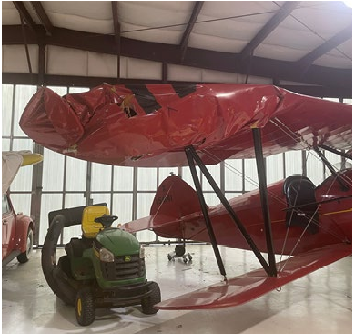
Photograph 2 - Right upper wing damage (Courtesy of FAA)
