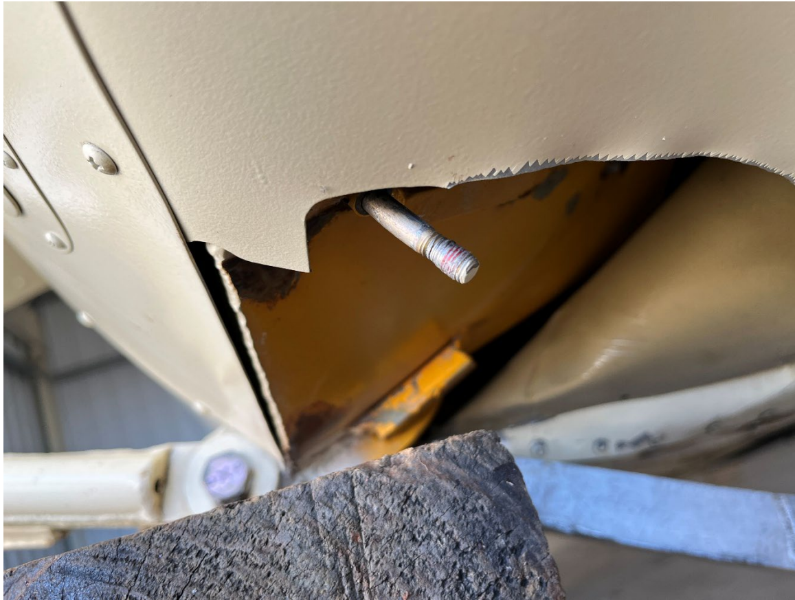
Photograph 7 - Gear leg retention bracket bolt with locknut threads (Courtesy of FAA)
