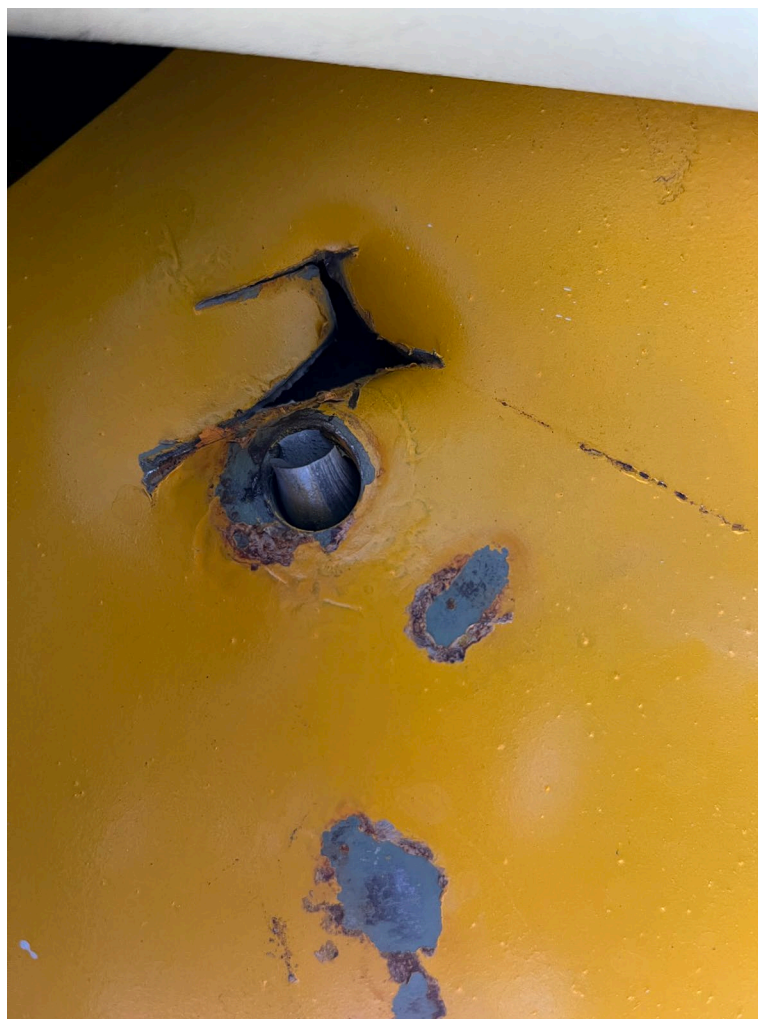
Photograph 4 - Postaccident damaged landing gear attach plate with bolt half (Courtesy of FAA)
