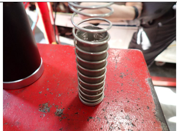
Image 9: Airframe fuel strainer screen
