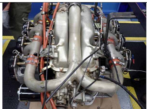
Photograph 2: Bottom of engine overview (impact damage to intake tube visible)
