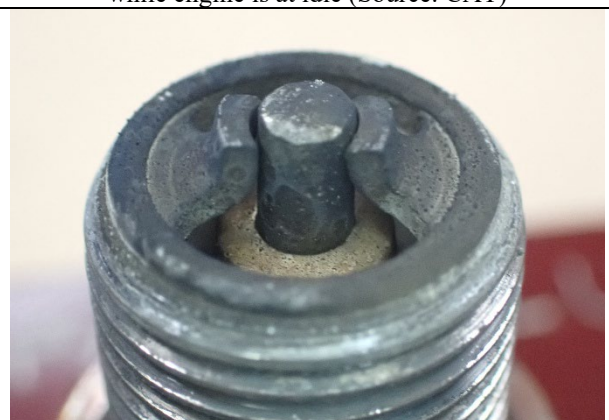
Photograph 8: No. 5 top spark plug found after initial engine run with no gap (Source: CAT)
