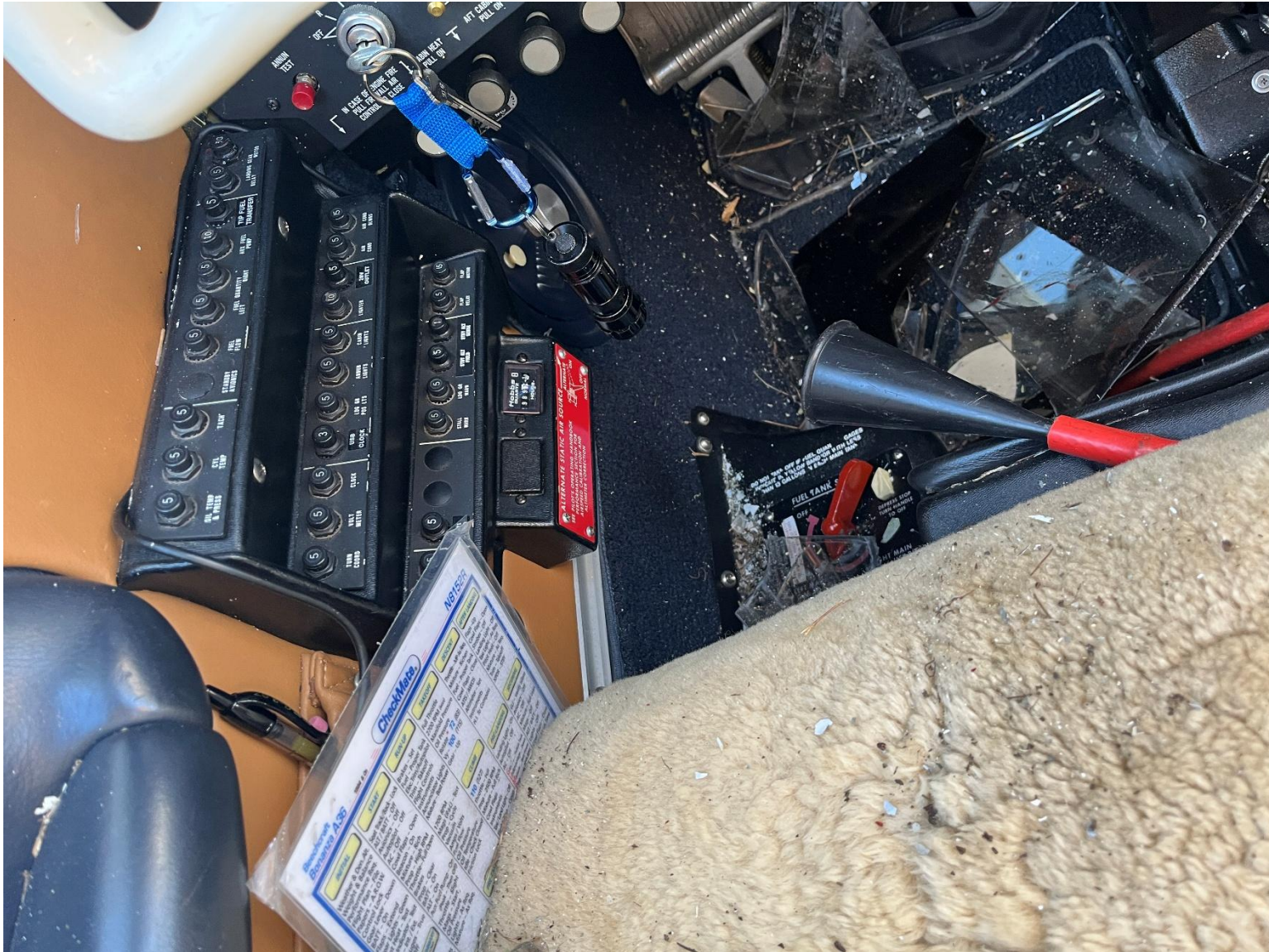
Photograph 6 - Cockpit image with fuel selector visible in the "LEFT" position (Source: FAA)
