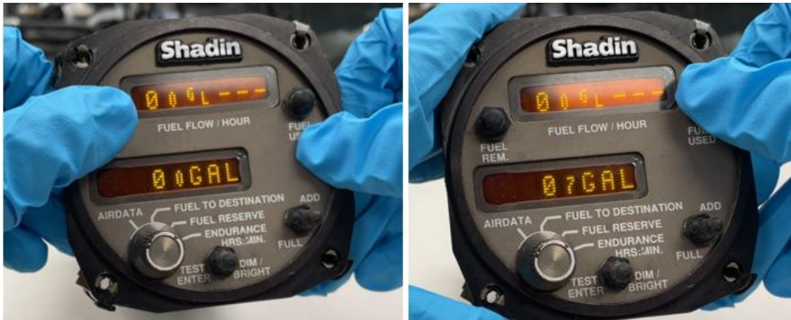
Figure 2. Shadin DigiData Fuel Remaining (left) at 0.0 gallons and Fuel Used (right) at 0.7 gallons.
