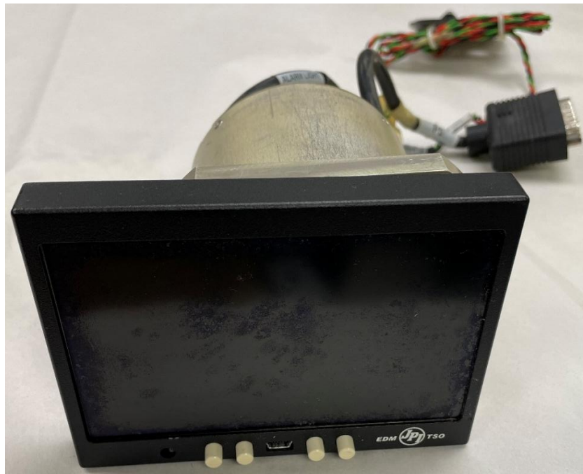
Figure 1. JPI EDM-900 as received by the NTSB Vehicle Recorder Laboratory.
