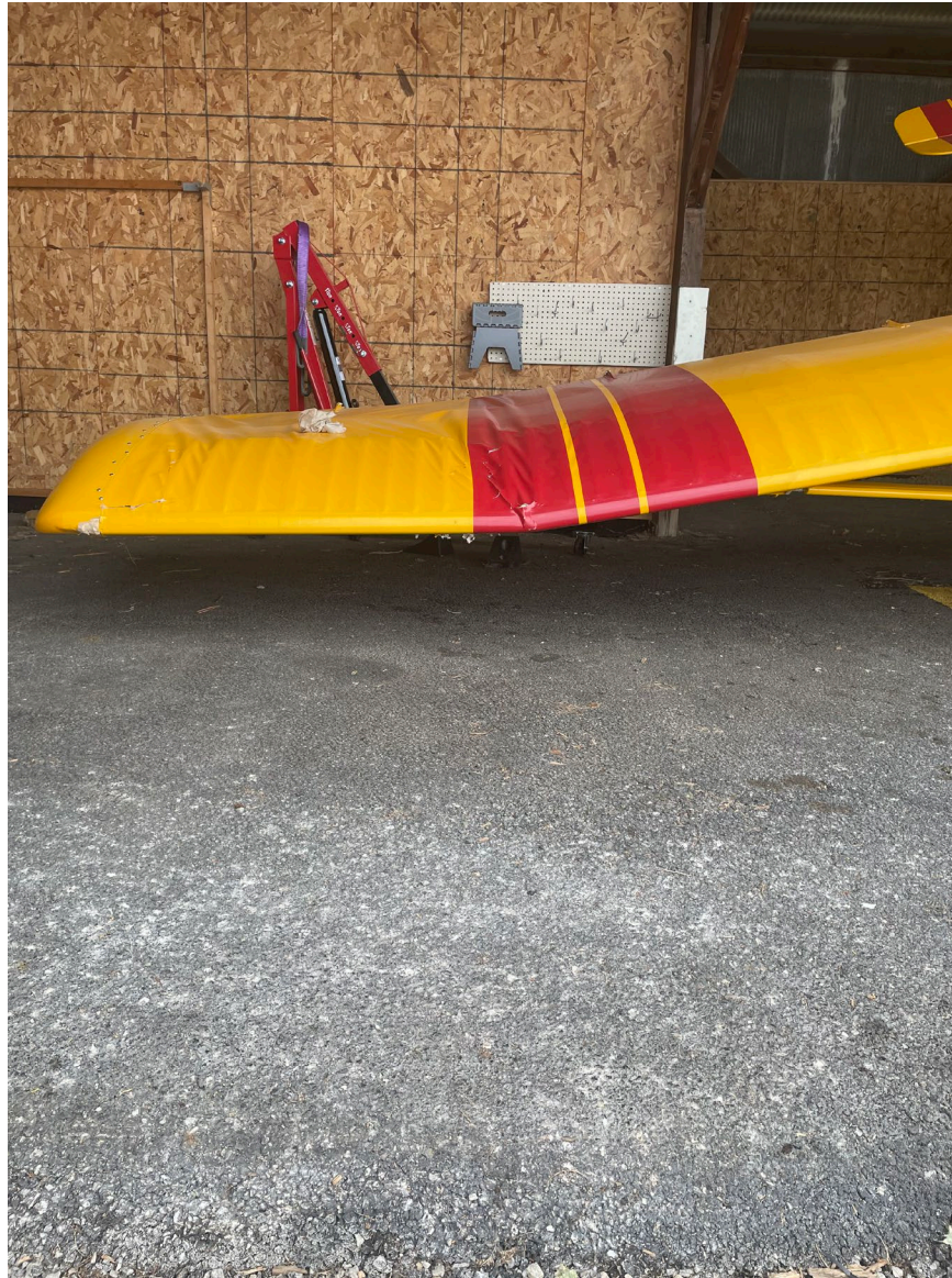
Photograph 2 - Deformation noted to right wing (Courtesy of FAA)
