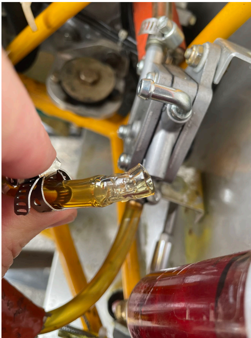
Photograph 3 - Split noted to fuel line (Courtesy of FAA)
