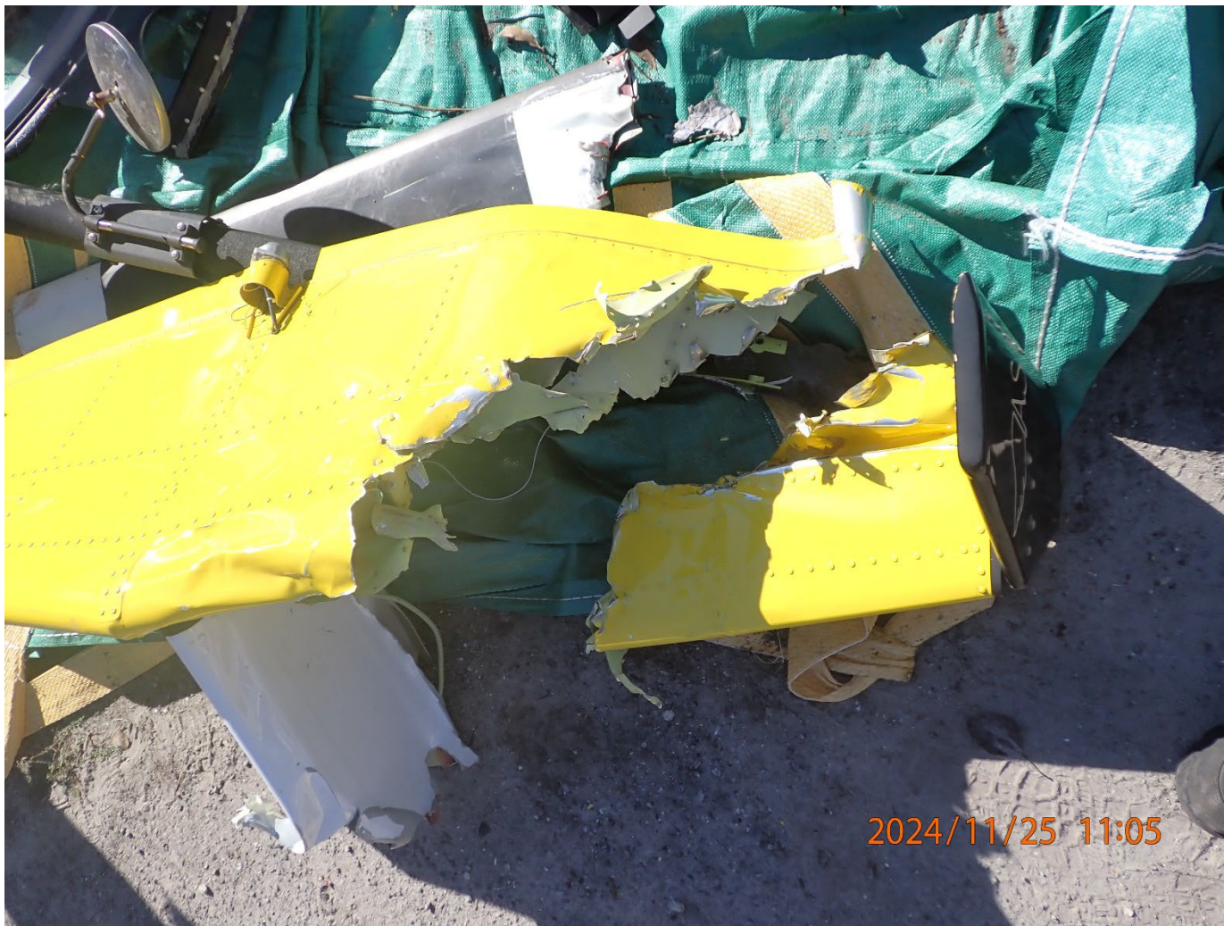
Photograph 1 - Cable damage to stabilizer. (NTSB)
