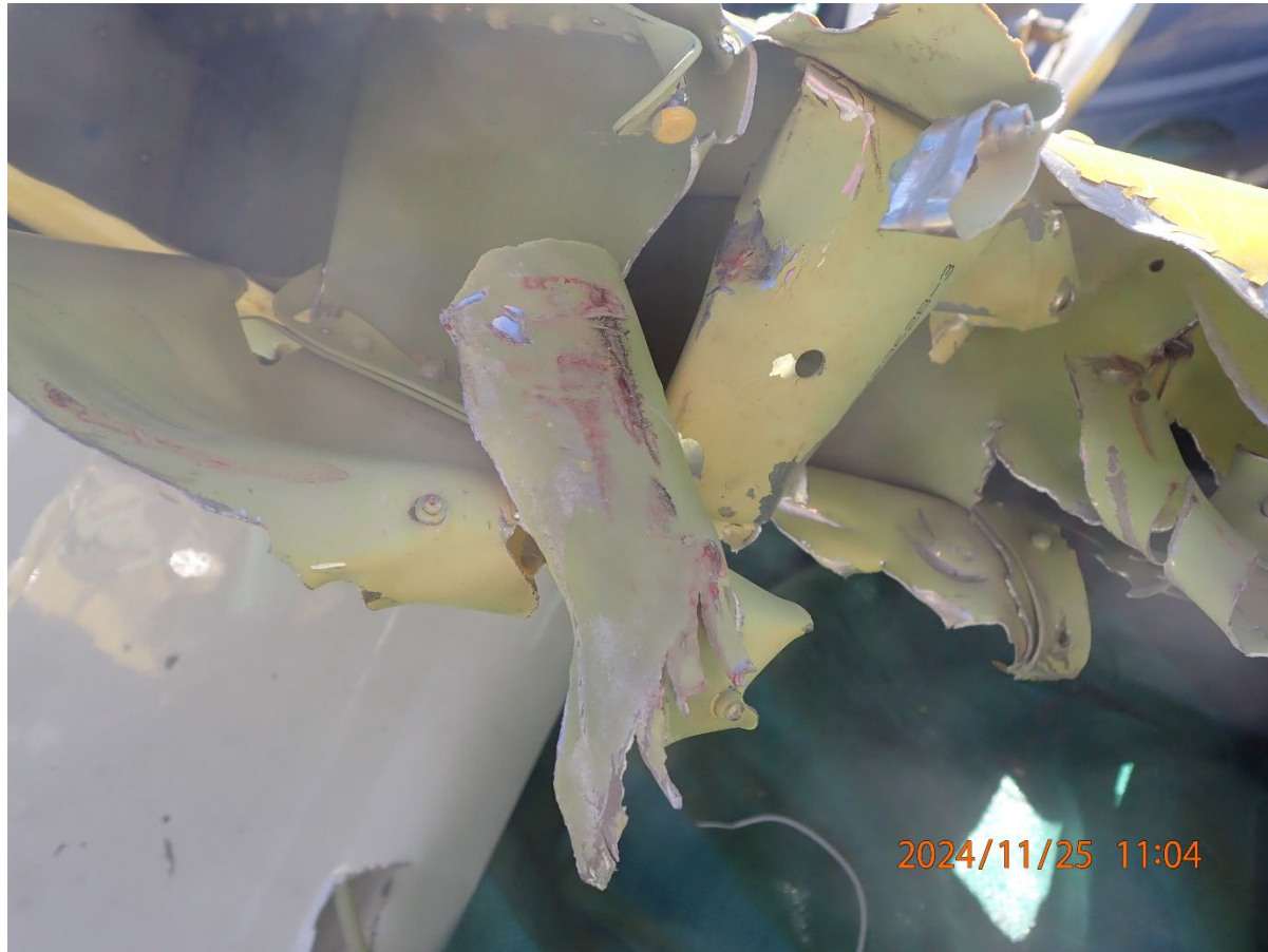
Photograph 2 - Cable striation marks in stabilizer. (NTSB)
