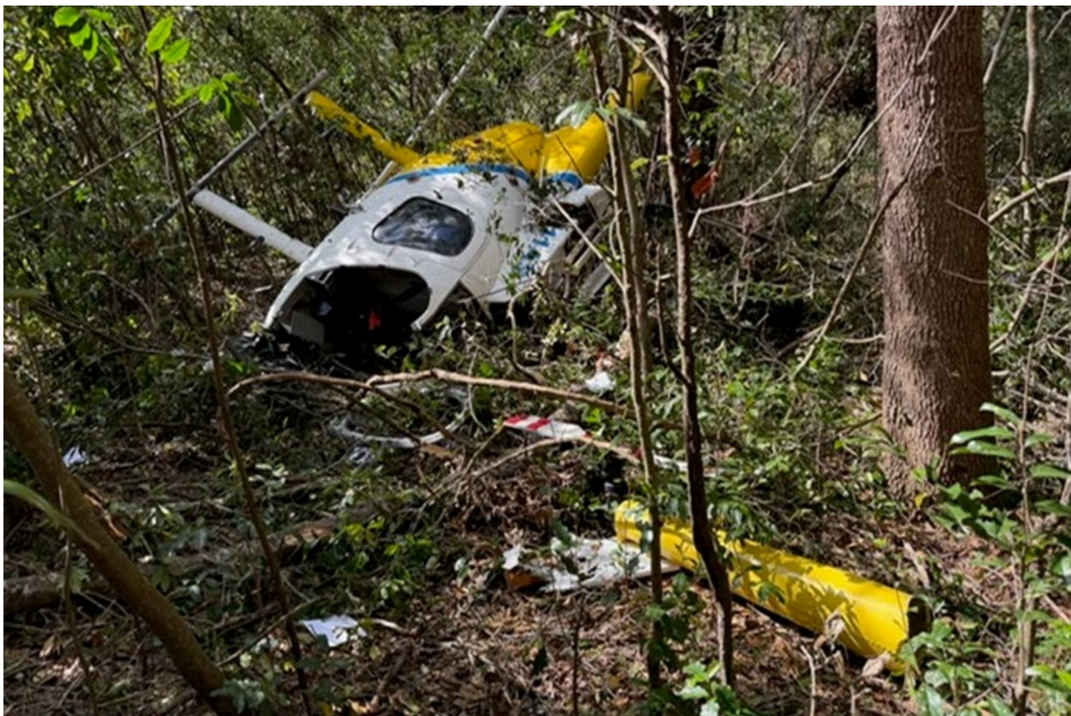
Photograph 1 - View of damaged helicopter and separated tail boom. (Courtesy of Operator)
