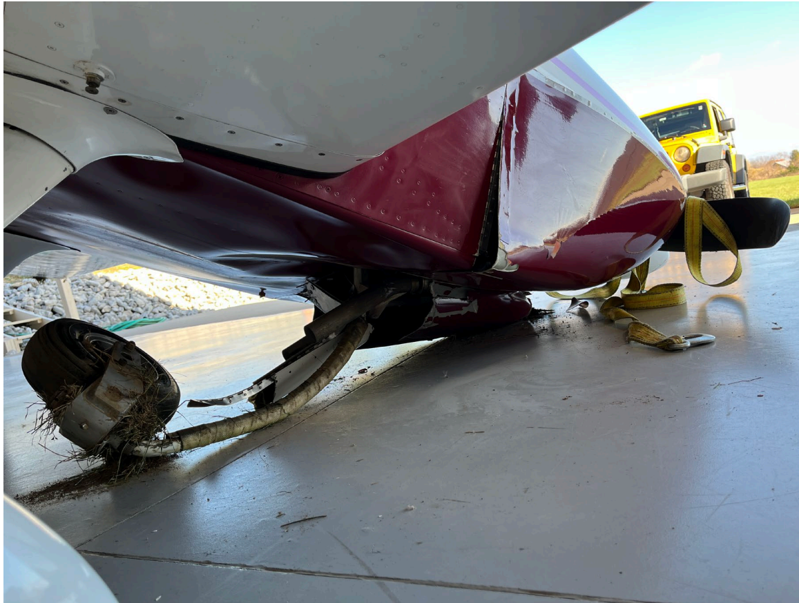
Photograph 2 - Lower fuselage accident damage, right side (Courtesy of FAA)
