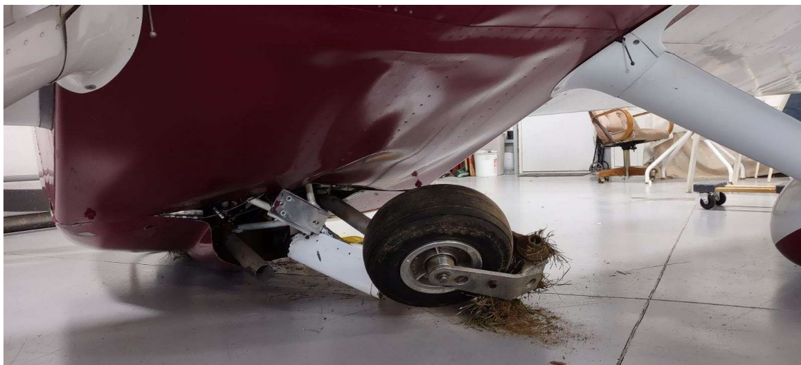
Photograph 1 - Lower fuselage accident damage (Courtesy of Pilot)
