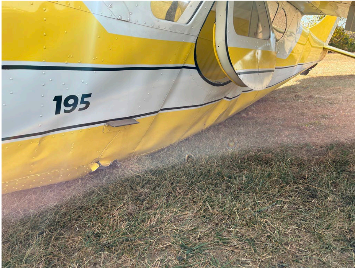
Photograph 4 - Fuselage Damage on Left Side of Airplane (Courtesy of FAA)
