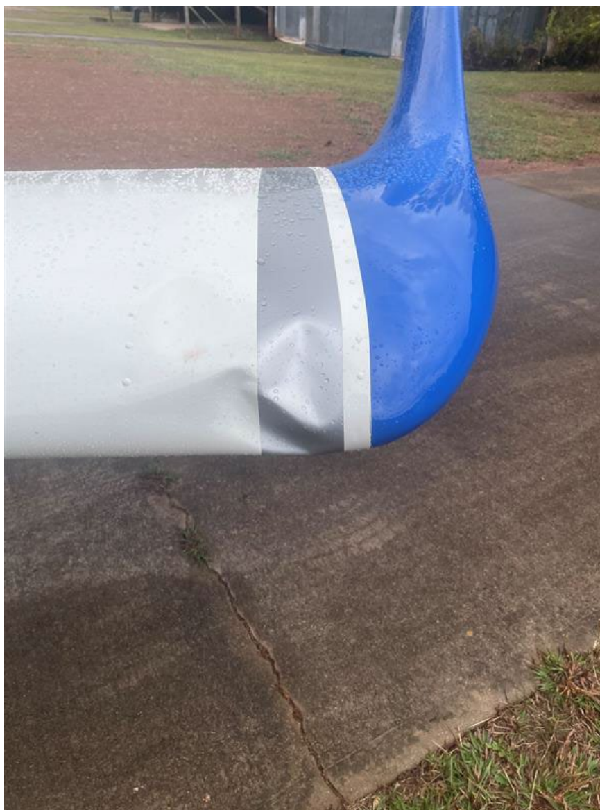
Photograph 1 - Skin deformation noted to outboard area of the left wing (Courtesy of FAA)
