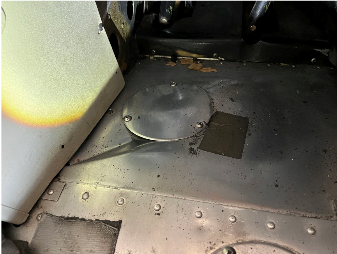
Photograph 4 - Floorboard wrinkling (Courtesy of FAA)
