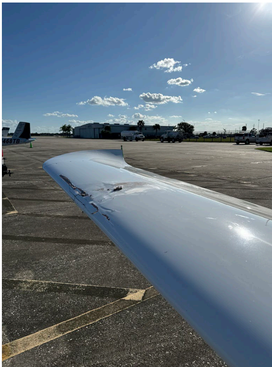
Photograph 1 - Left Side View of Right Wing Damage (Courtesy of FAA)
