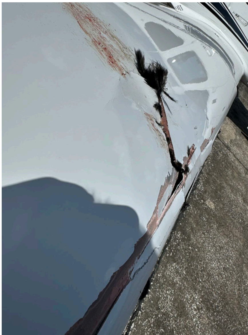
Photograph 2 - Right Side View of Right Wing Damage (Courtesy of FAA)
