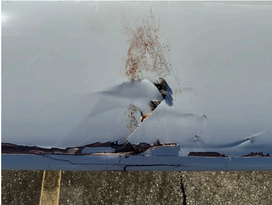
Photograph 3 - Closeup View of Right Wing Damage (Courtesy of FAA)
