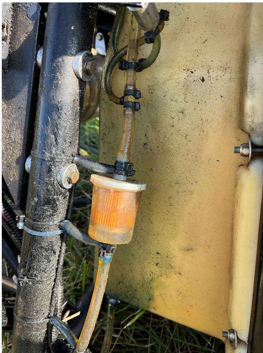
Photo 14: View of the inline fuel filter with fuel still in the bowl and line. (Courtesy of FAA)
