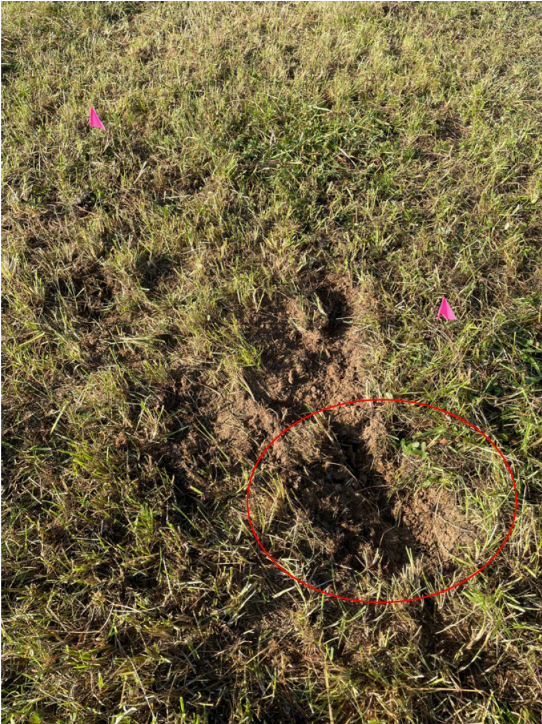
Photo 5: Nose gear impact ground scar (circled). (Courtesy of FAA)
