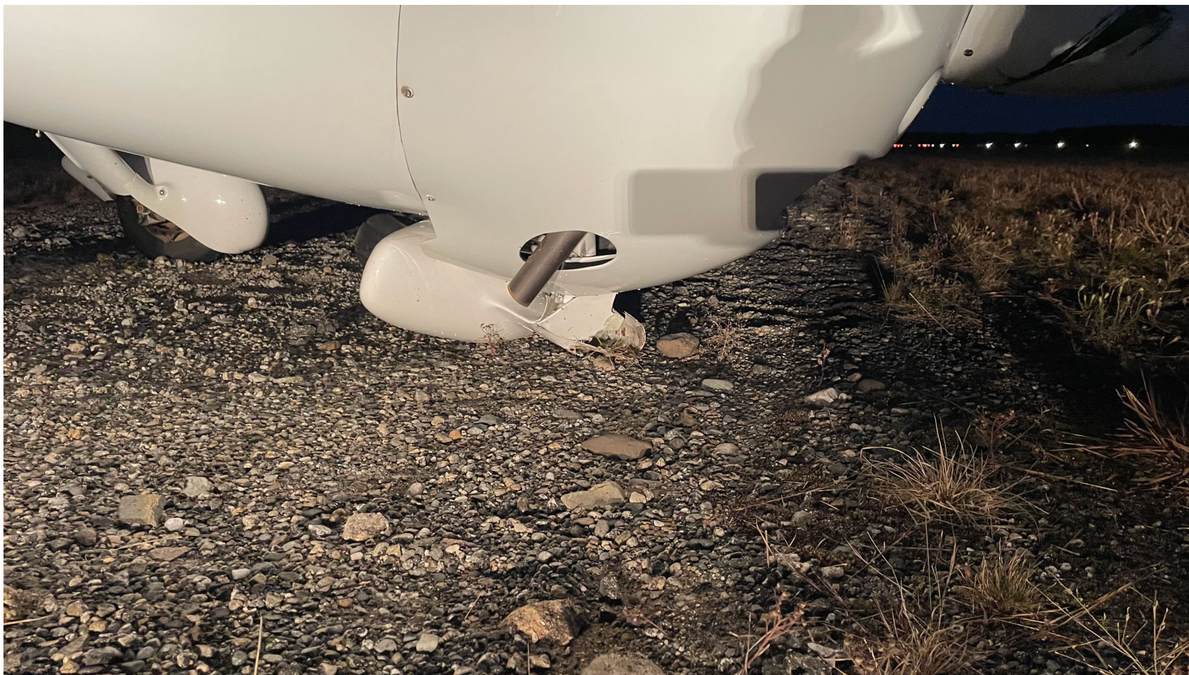
Photograph 2 - Buckled Nose Landing Gear (Courtesy of FAA)
