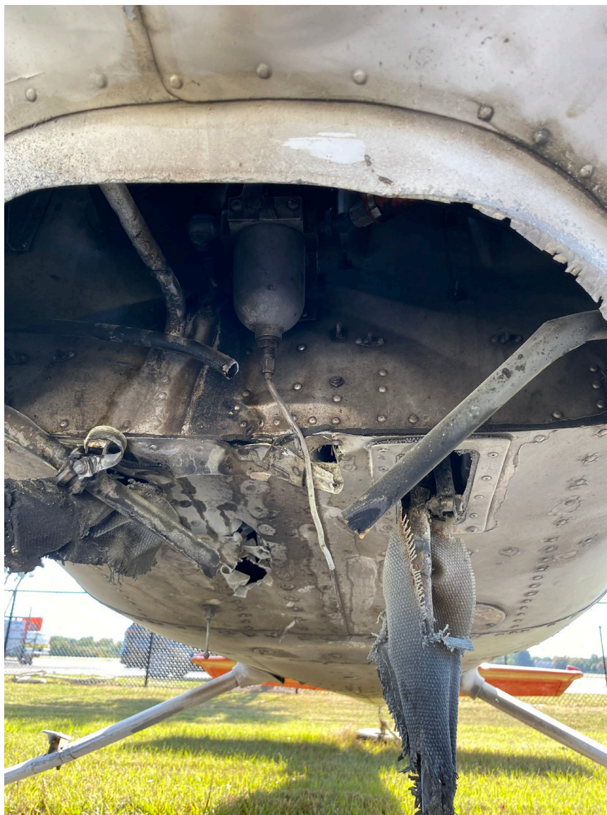
Photograph 3 - Substantial Damage to Engine Mount and Forward Fuselage Structure (Courtesy of FAA)
