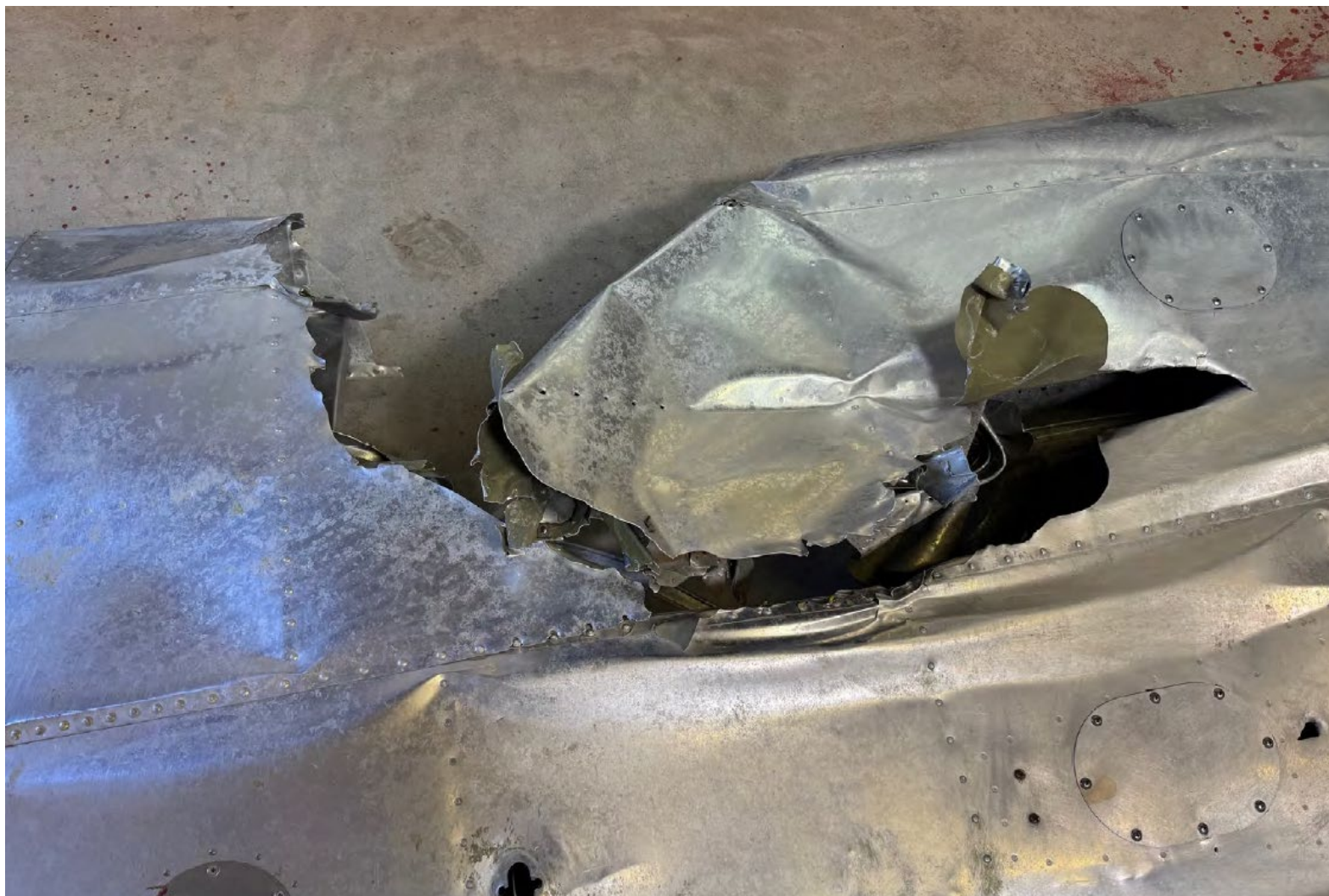
Photograph 4 - Left wing damage from pole. (Courtesy of Leading Edge Investigations)
