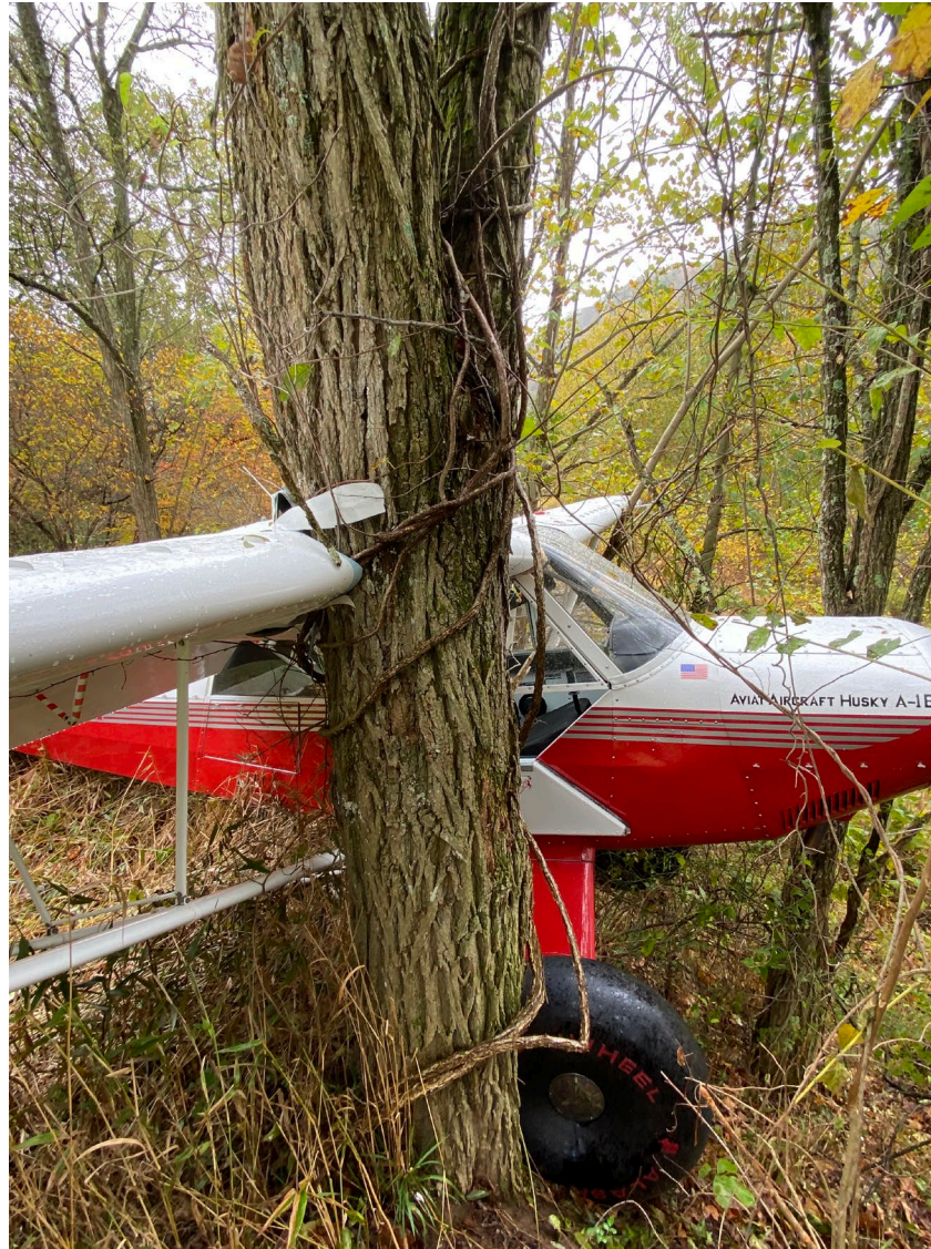
Photograph 1 - FAA Digital Photograph. Right Side View of the Airplane At the Accident Site. Note the Large Tree Contact to the Leading Edge Near the Wing Root
