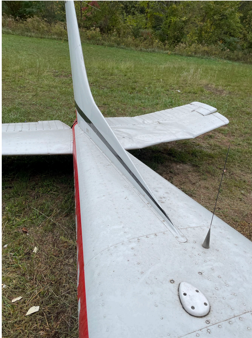
Photograph 3 - Damage to the Left Elevator (Courtesy of FAA)
