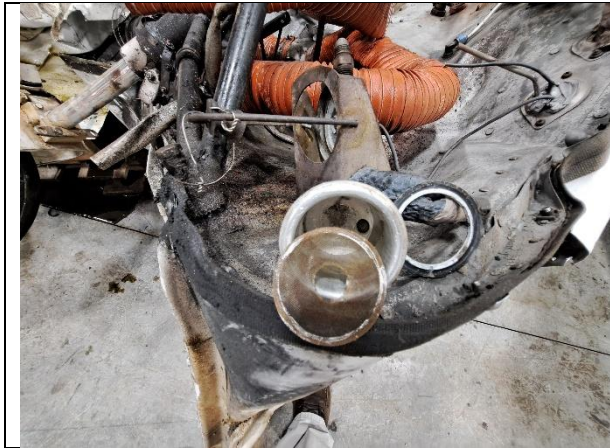
Photograph 7: Fuel strainer and screen (Source: Piper Aircraft)
