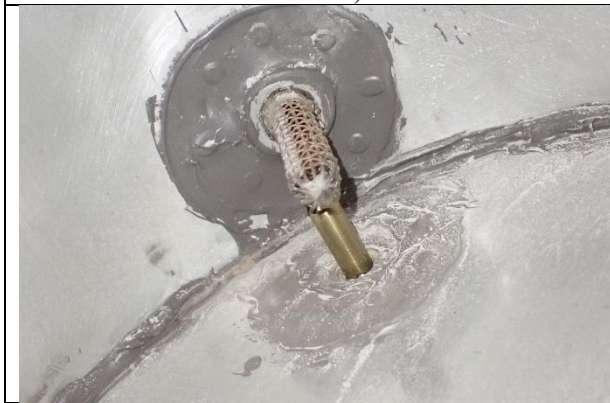
Photograph 9: Left fuel tank pickup screen (Source: NTSB)
