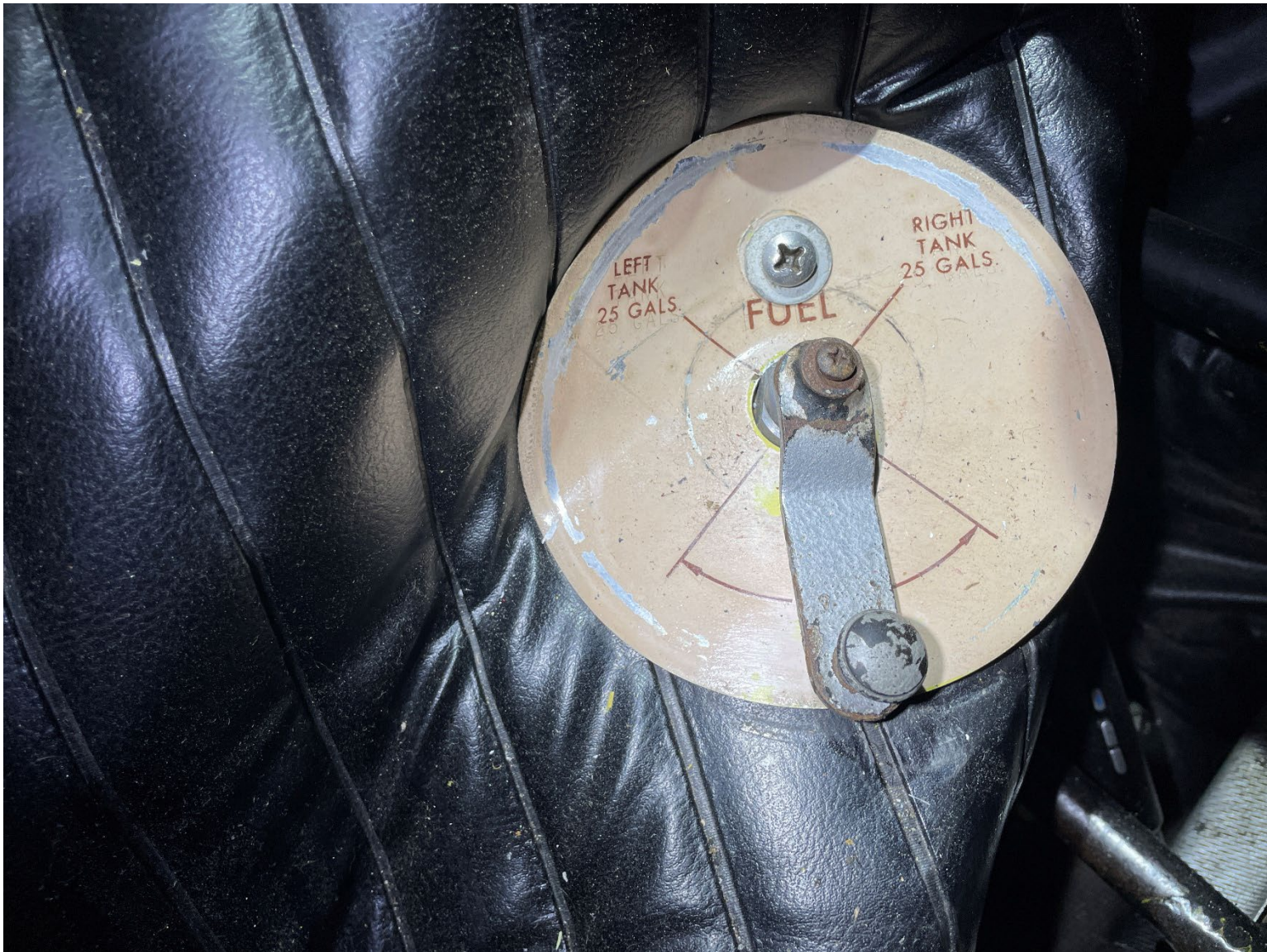
Photograph 5 - Fuel selector handle as found after initial recovery (Courtesy of FAA)
