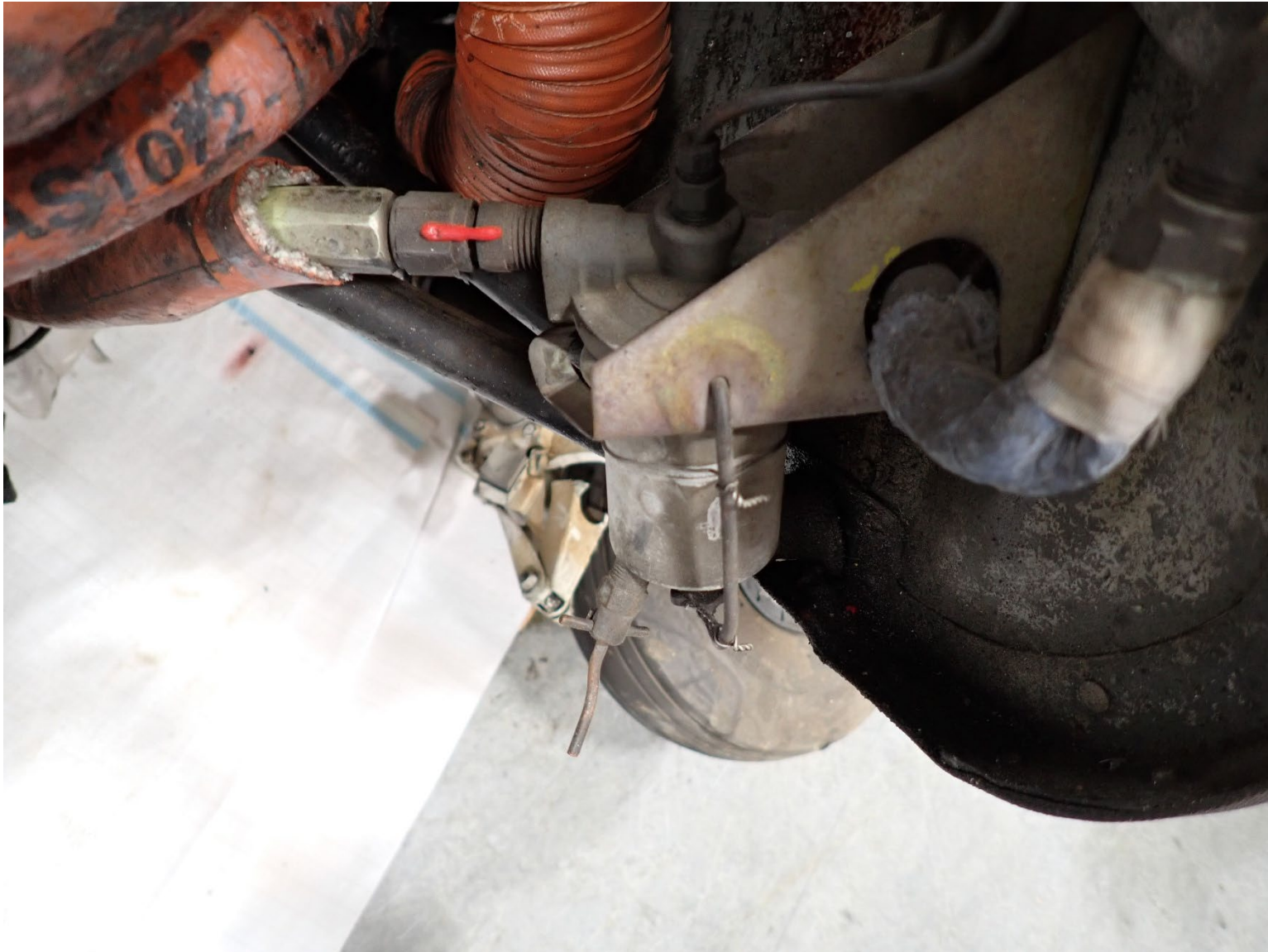
Photograph 10 - Fuel strainer and fuel line
