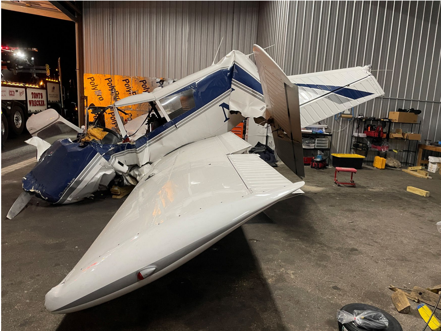
Photograph 3 - Airplane after initial recovery (Courtesy of FAA)
