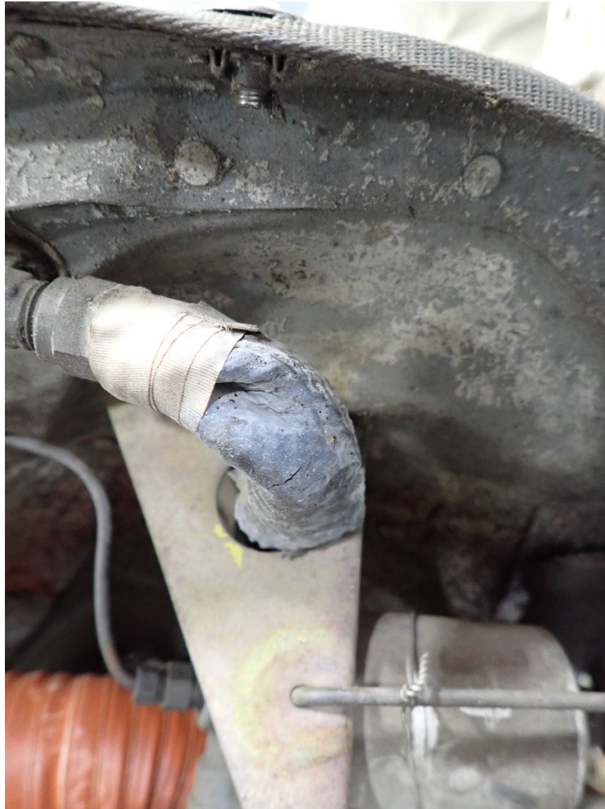
Photograph 11 - Fuel line going from firewall to fuel strainer
