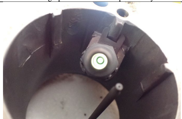
Photograph 4: Main nozzle with light passing through the passage
