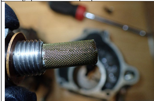
Photograph 9: Fuel inlet screen
