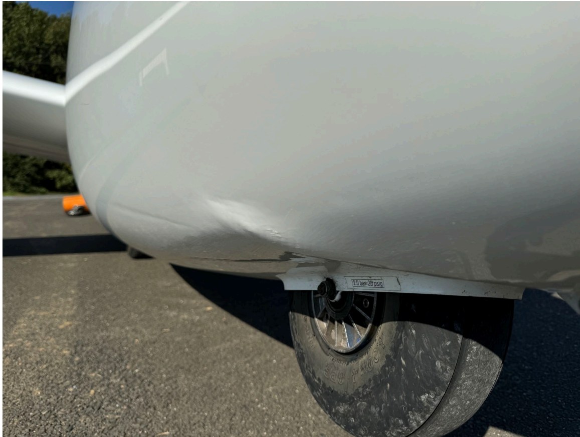
Photograph 3 - Fuselage damage (Courtesy of Pilot)
