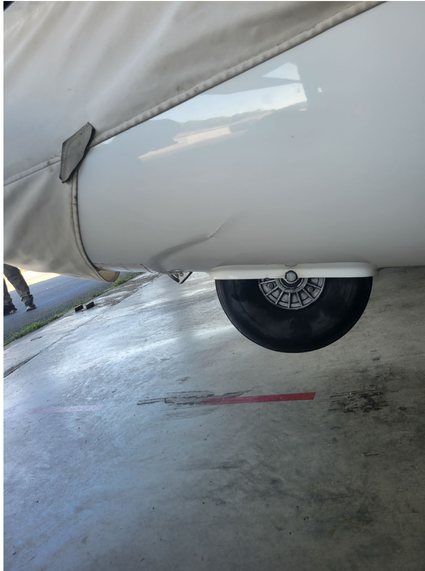
Photograph 2 - Fuselage damage (Courtesy of Pilot)
