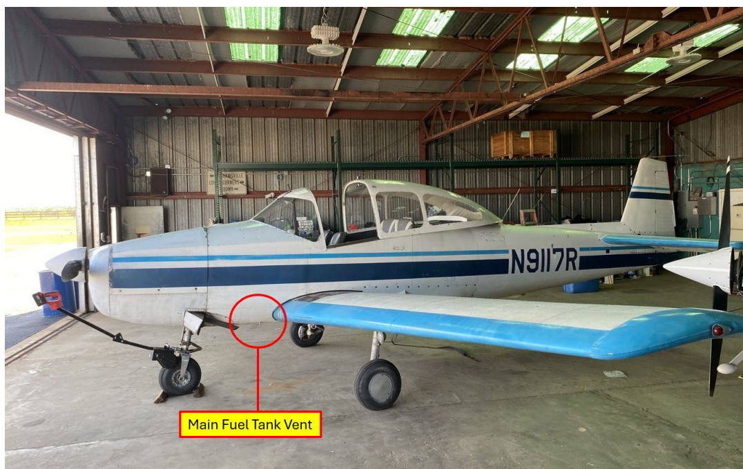
Figure 2- Annotated photograph of the vent location.
