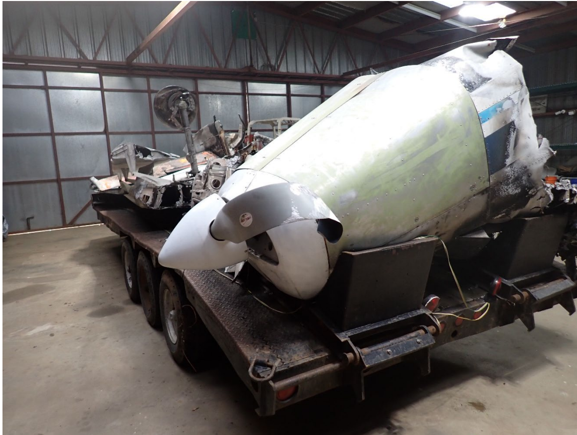
Photograph 3 - Thermally separated nose section (NTSB)
