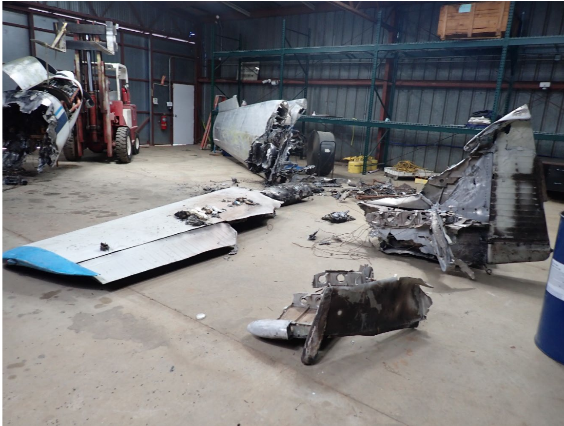
Photograph 2 - Thermally destroyed fuselage (NTSB)
