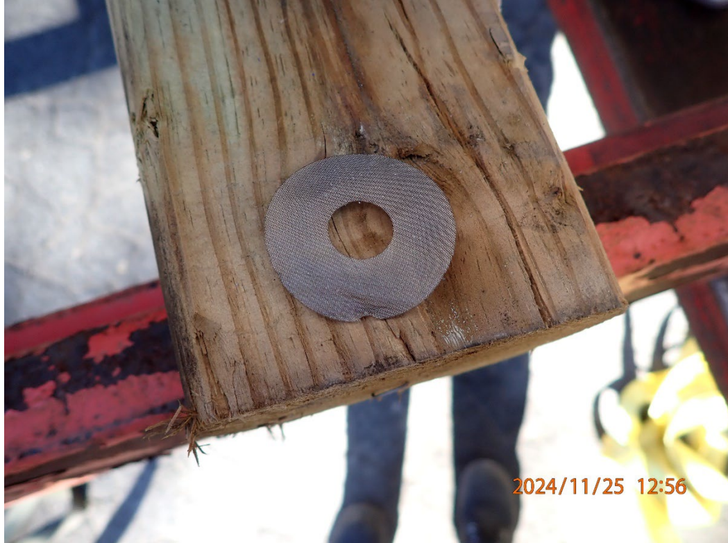
Photo 6: View of the unobstructed fuel strainer screen.
