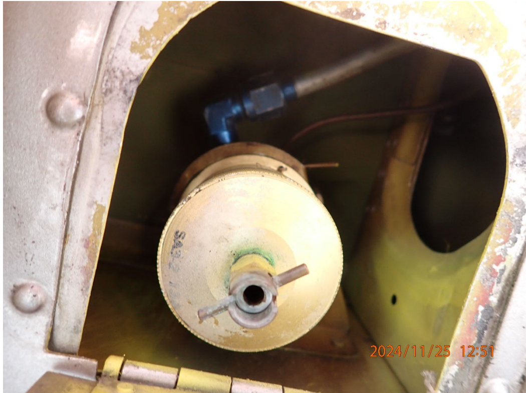
Photo 4: View of the fuel strainer.
