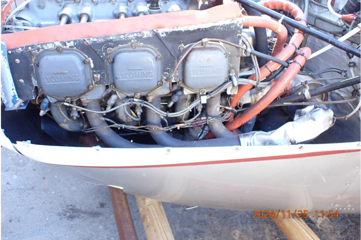
Photo 3: View of the undamaged exhaust.
