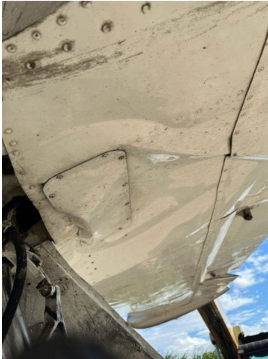
Photograph 2 - Right Wing Damage (Courtesy of FAA)
