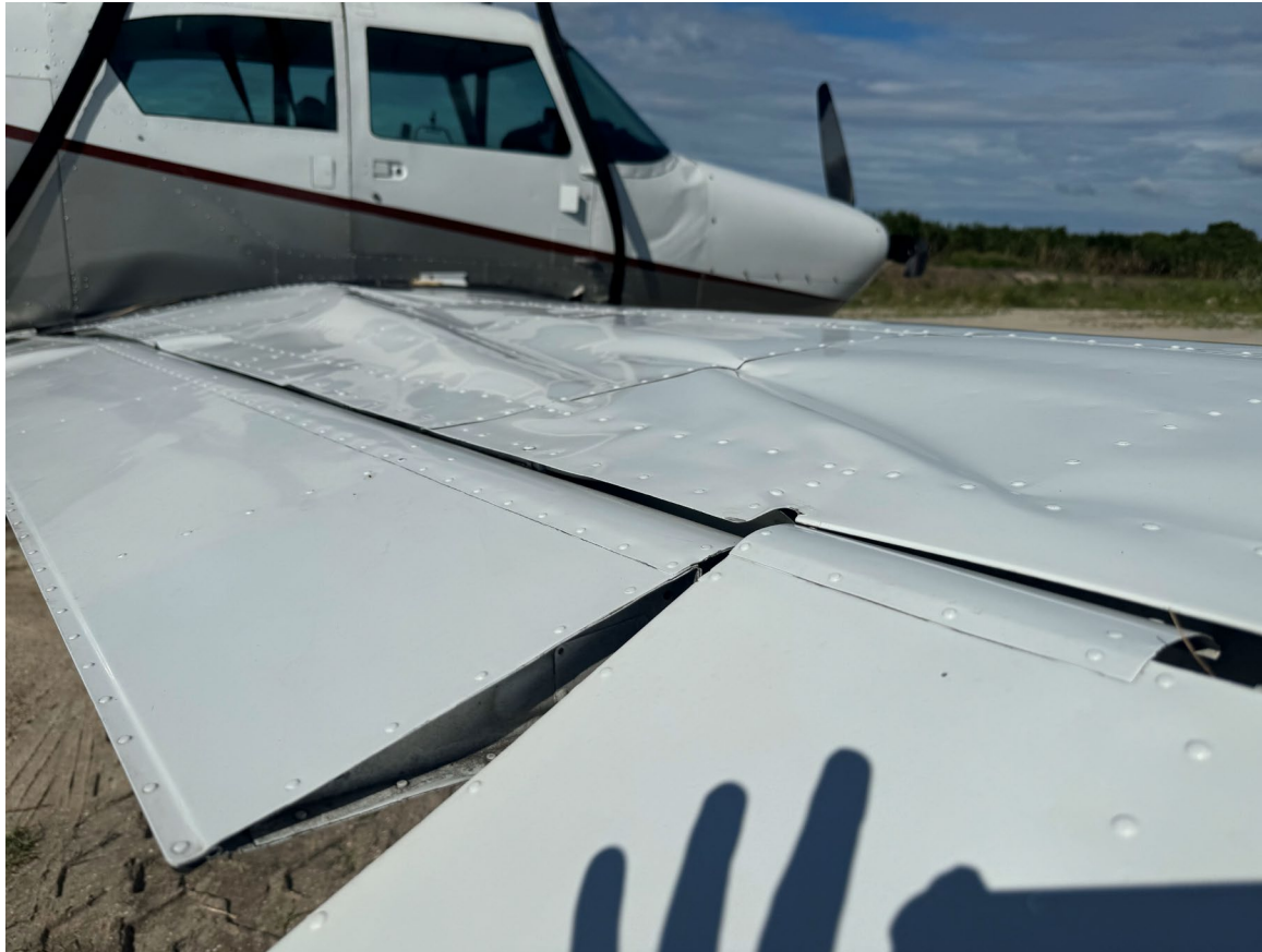
Photograph 3 - Right Wing Damage (Courtesy of FAA)
