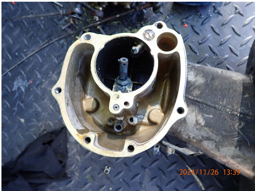
Photo 30: View of the carburetor bowl after the removal of the liquid.
