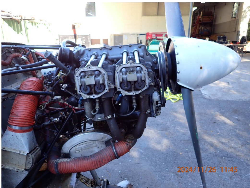
Photo 19: View of the Nos. 1 & 3 cylinders with rocker box covers removed.
