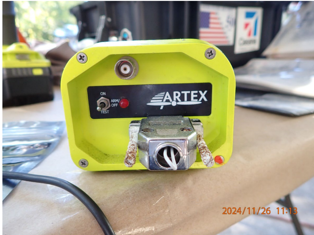
Photo 16: View of the front of the ELT.
