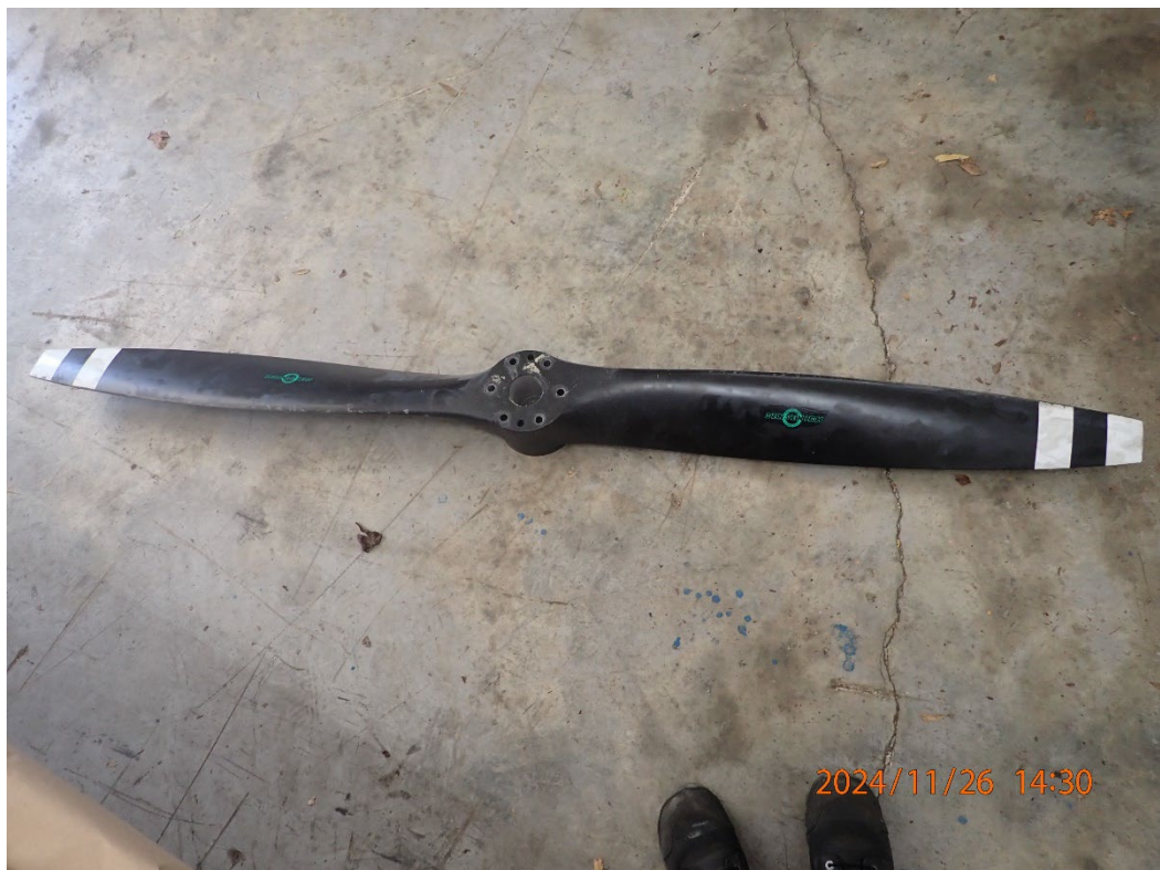
Photo 36: View of the undamaged propeller removed from the airplane.
