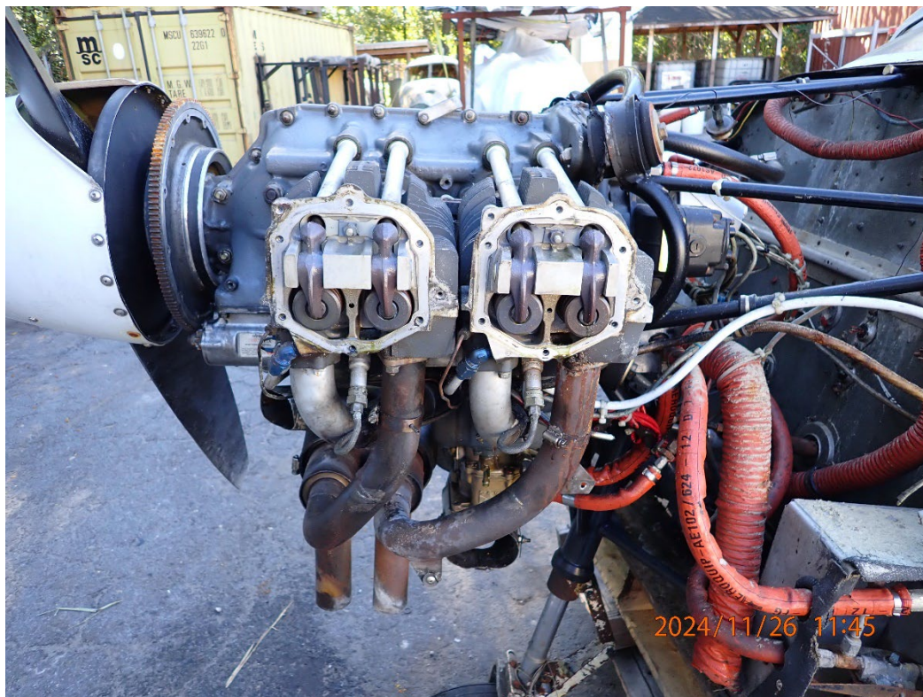
Photo 18: View of the Nos. 2 & 4 cylinders with rocker box covers removed.
