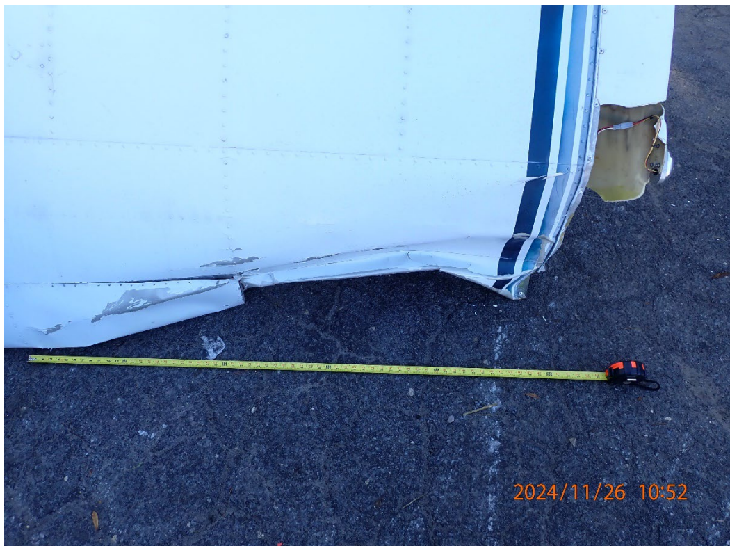
Photo 8: View of damage to the leading edge of the left wing.
