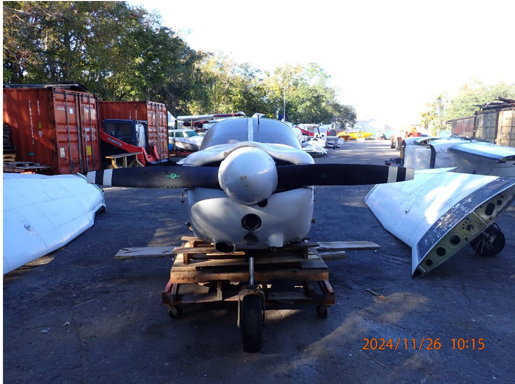
Photo 35: View of the undamaged propeller attached to the airplane.
