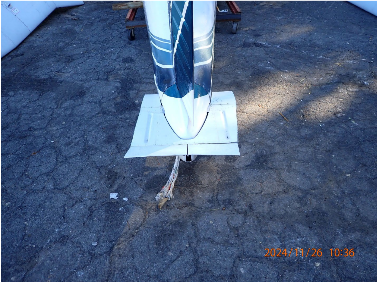
Photo 3: View of the remaining portions of the stabilator and stabilator trim.
