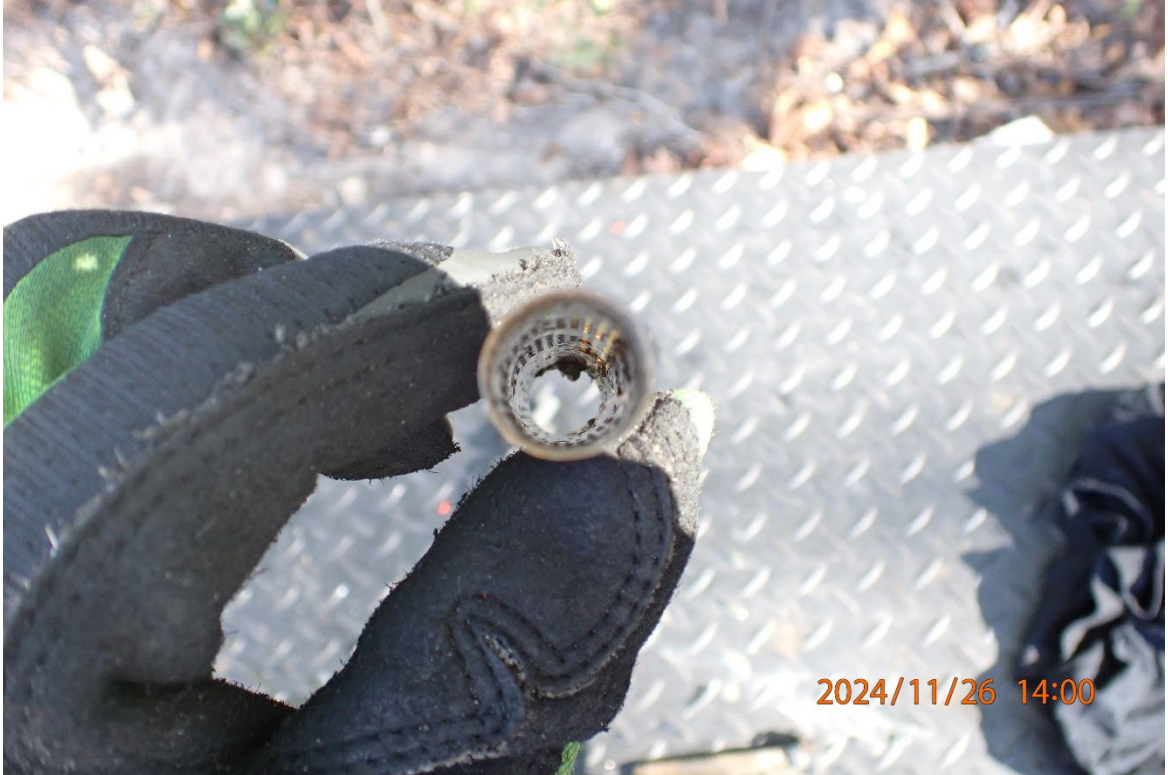
Photo 32: View of the oil suction screen.
