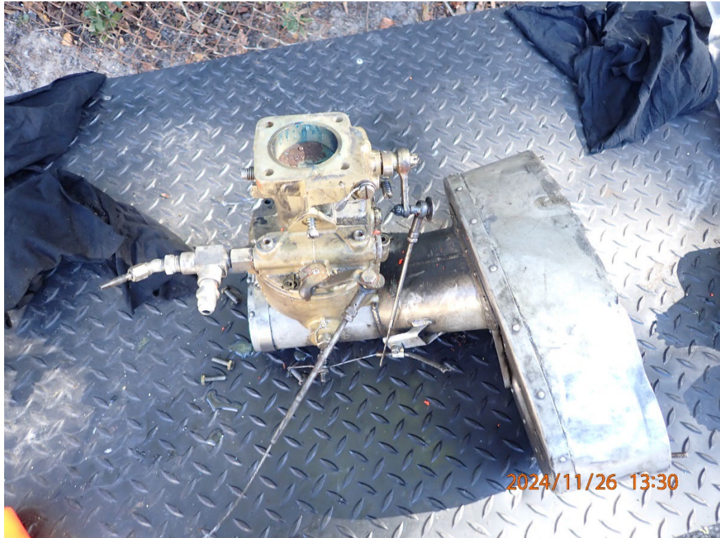
Photo 27: View of the carburetor removed from the engine.
