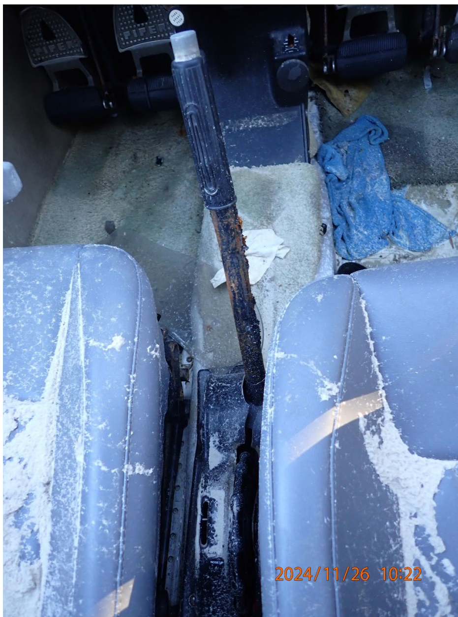
Photo 9: View of the stabilator trim control and flap control handle.
