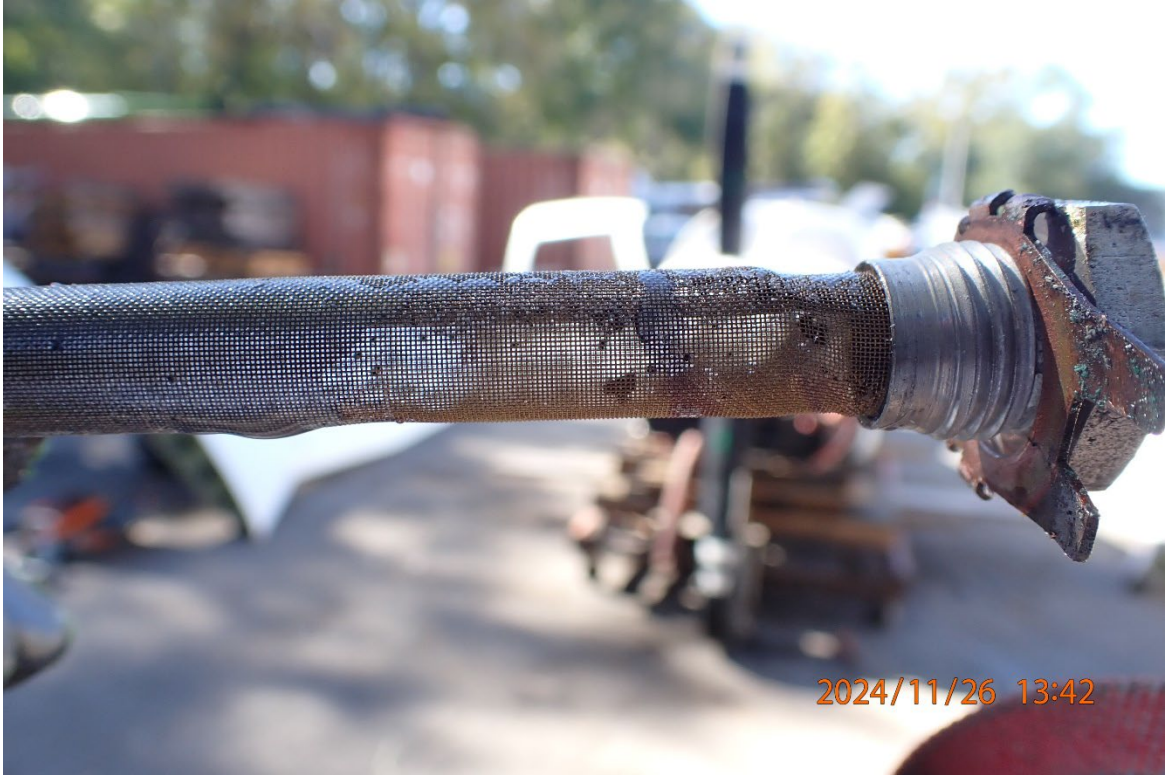
Photo 31: View of the carburetor fuel inlet screen.
