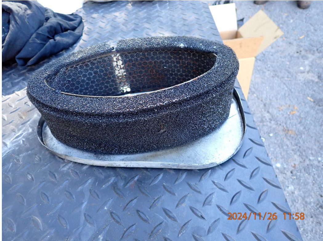
Photo 20: View of the unobstructed engine air filter.
