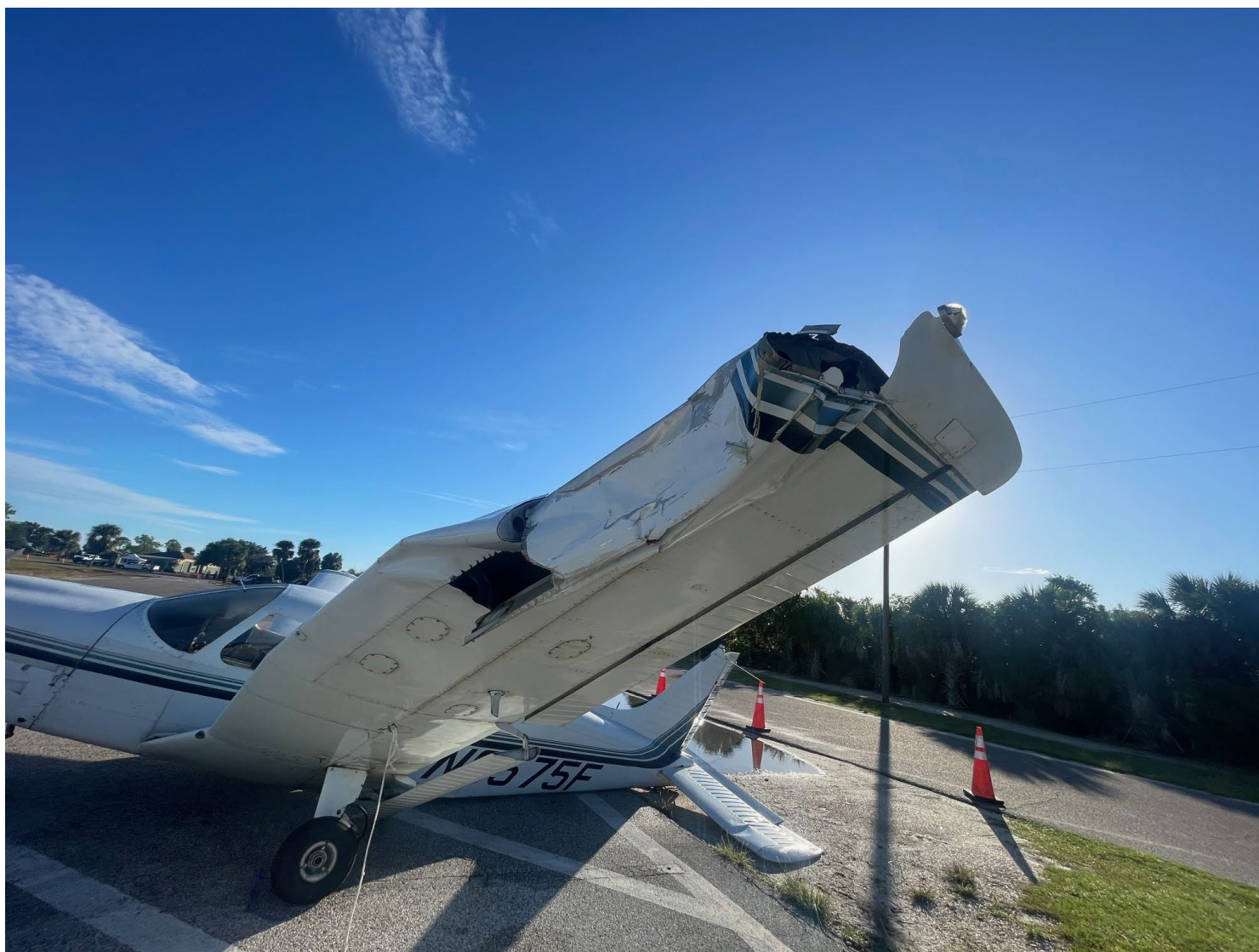
Photograph 2 - View of damage to the left wing. (Courtesy of Florida Air Recovery)
