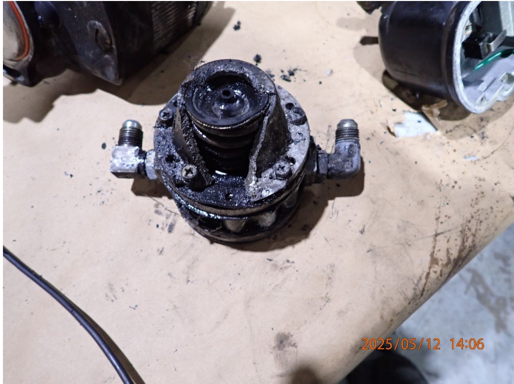
Photo 29: View of the engine driven fuel pump.
