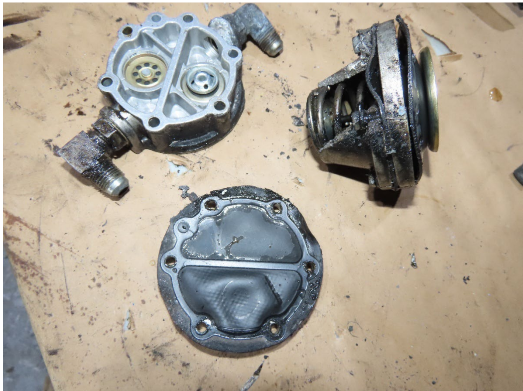
Photo 30: View of the disassembled engine driven fuel pump. (Courtesy of Lycoming)
