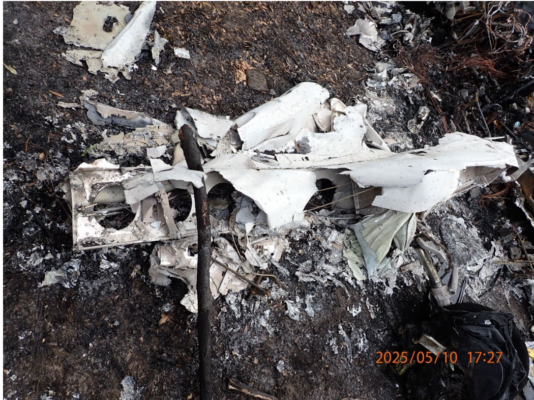
Photo 10: View of the inboard portion of the left wing.
