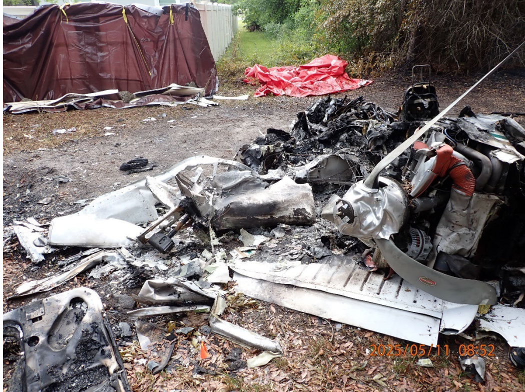
Photo 8: View of the remaining stabilator under the engine.
