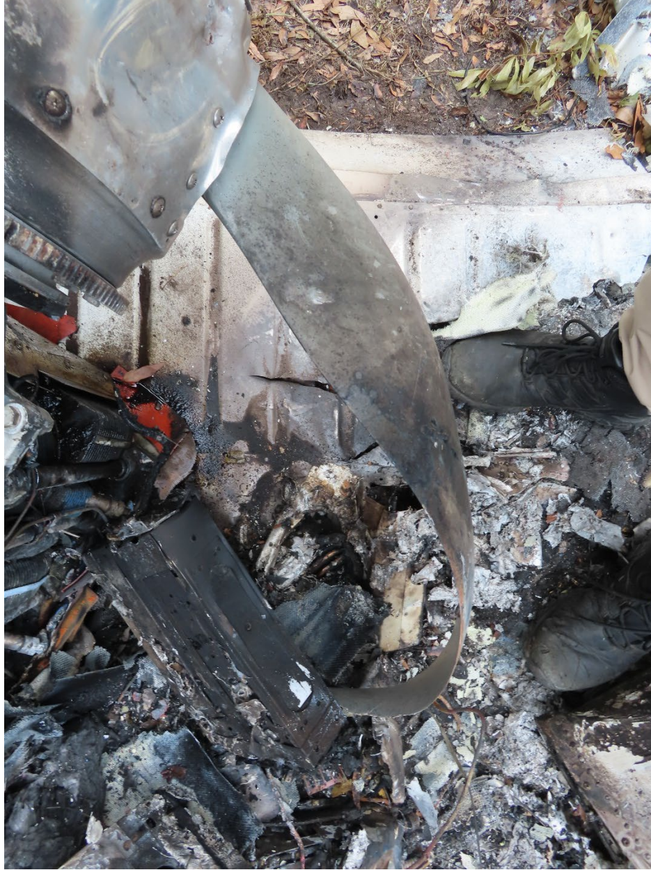
Photo 41: View of propeller blade aft bending. (Courtesy of Piper)
