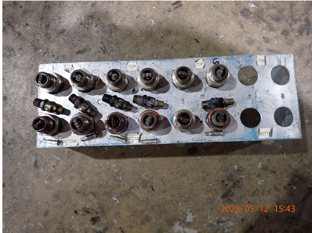
Photo 28: View of the spark plugs and fuel injectors.
