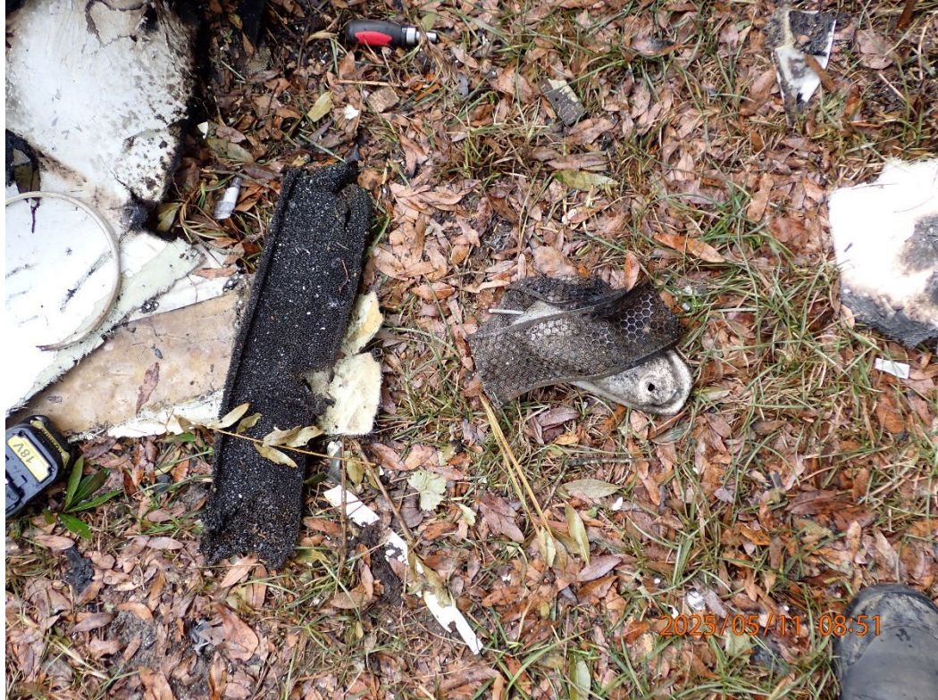
Photo 24: View of the remnants of the induction air filter.
