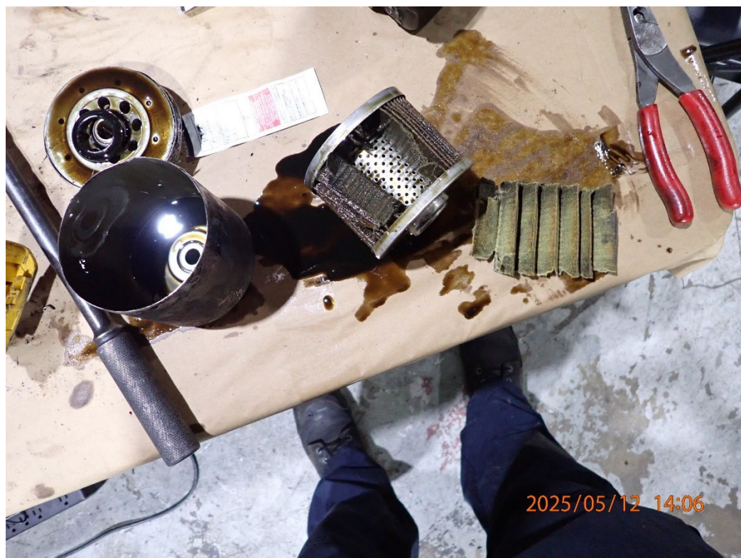
Photo 36: View of the cut open oil filter and unobstructed pleats.
