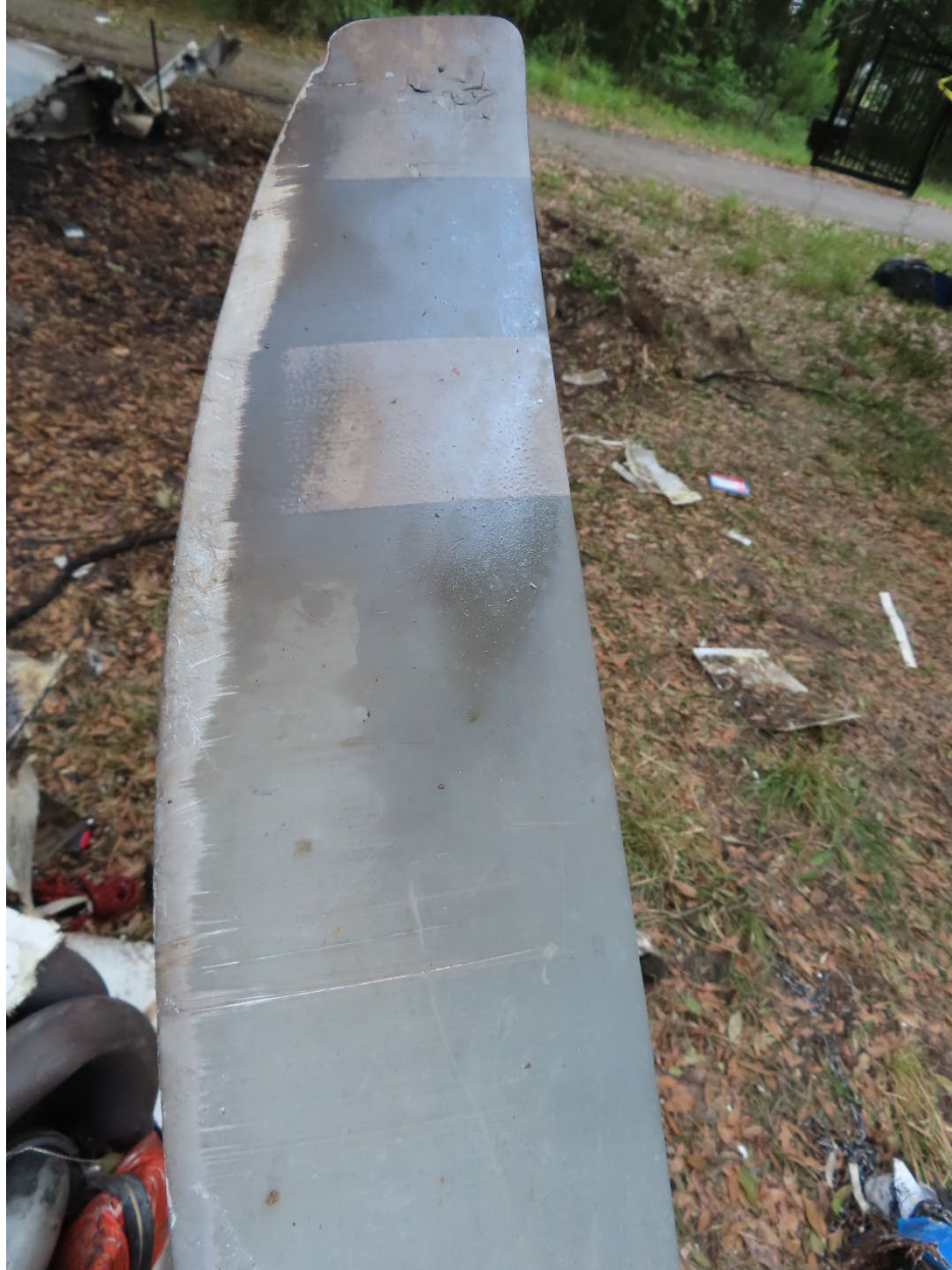
Photo 40: Propeller leading-edge polishing and gouging, and chordwise scratching. (Courtesy of Piper)
