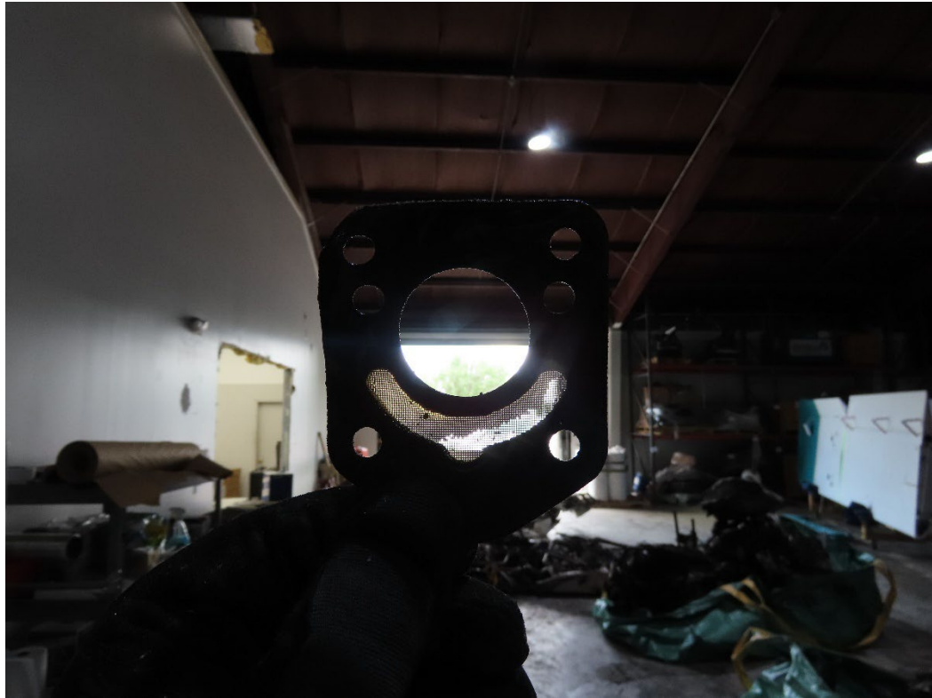
Photo 44: View of the unobstructed governor oil screen. (Courtesy of Lycoming)
