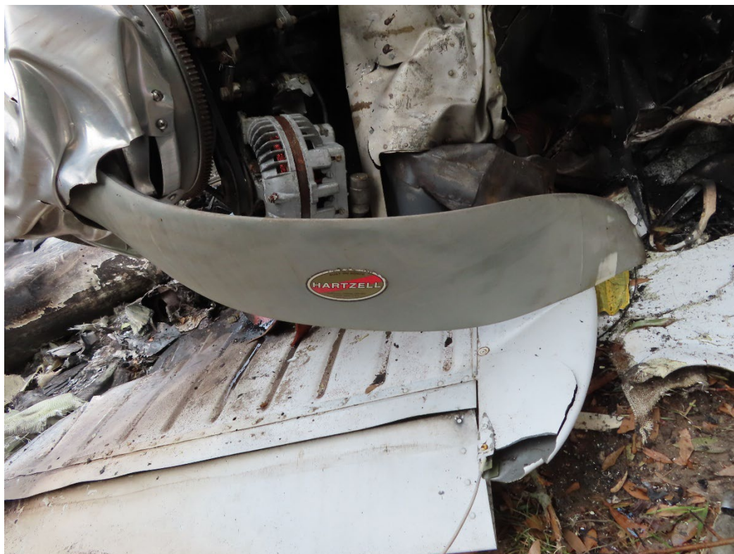
Photo 42: View of propeller blade aft bending. (Courtesy of Piper)
