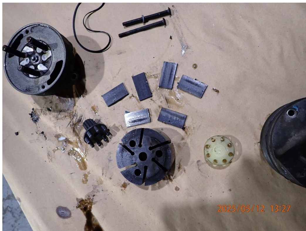
Photo 38: View of the disassembled vacuum pump.
