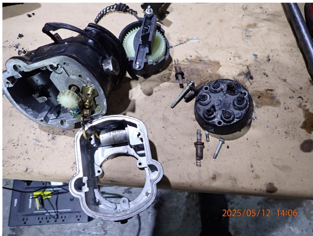
Photo 27: View of the disassembled left magneto.
