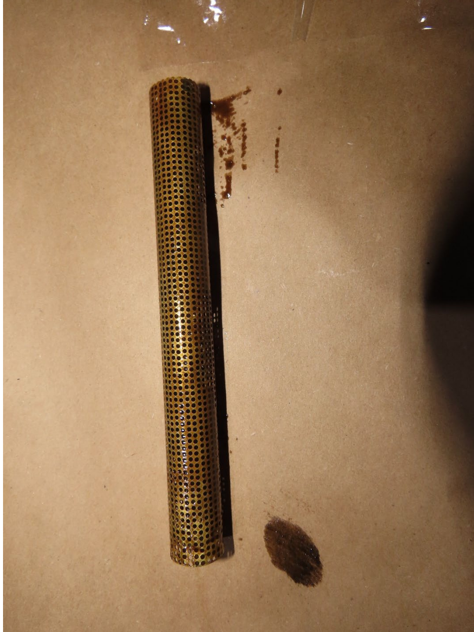
Photo 37: View of the unobstructed oil suction screen. (Courtesy of Lycoming)
