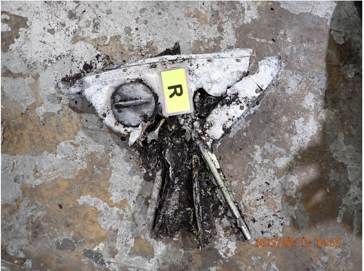
Photo 20: View of the right fuel tank cap.
