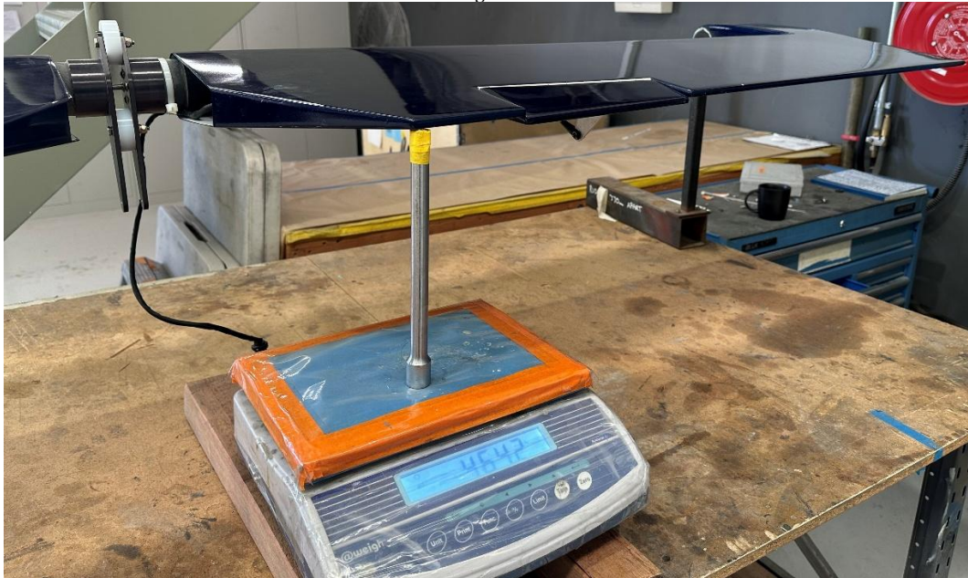
Elevator resting on the scales indicating trailing edge heavy weight
