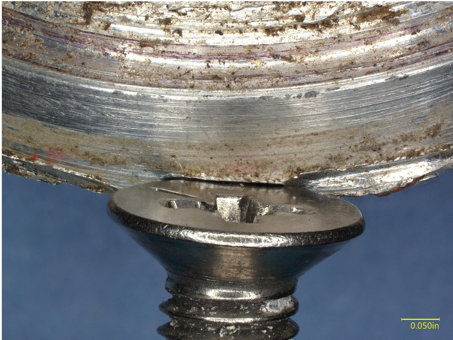
Photograph 5 - Close up of screw impression on plug
