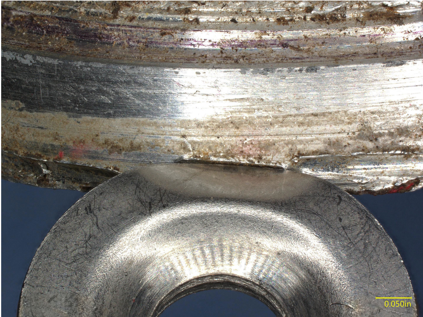
Photograph 4 - Close up of washer impression on plug
