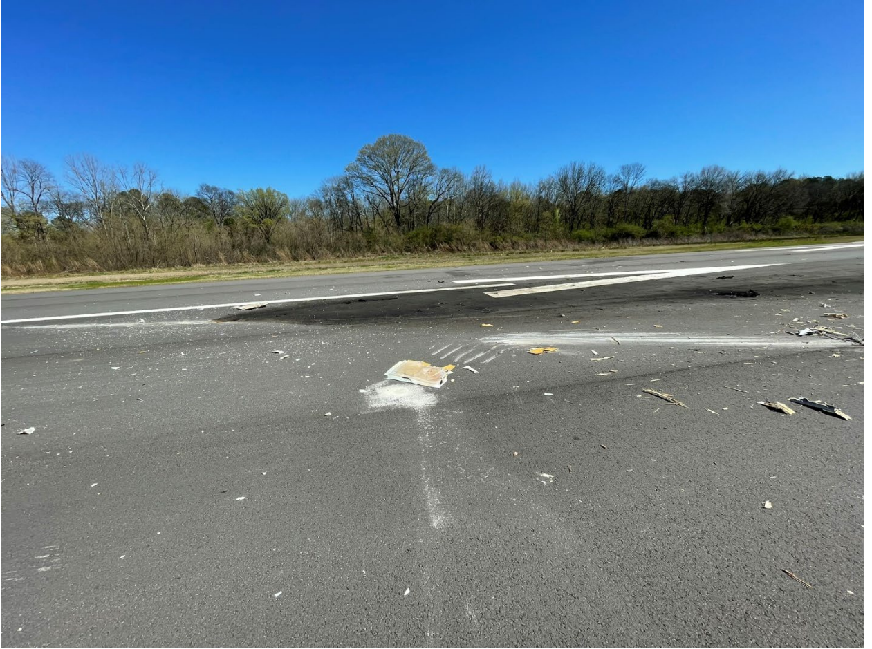
Figure 1: View of the propeller strike marks along the wreckage path.
