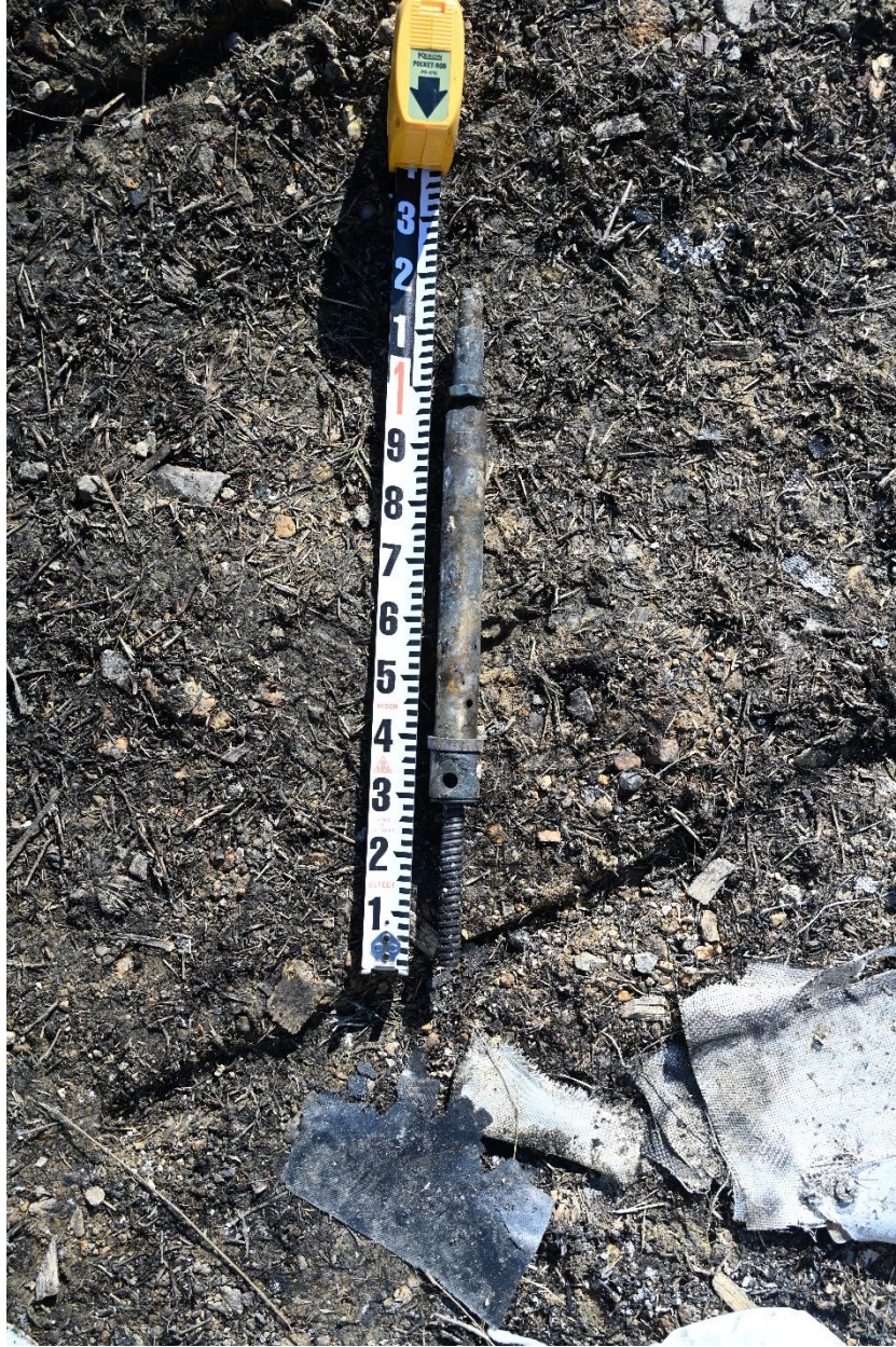
Photo 9: View of flap jackscrew with scale. (Cirrus Photo)
