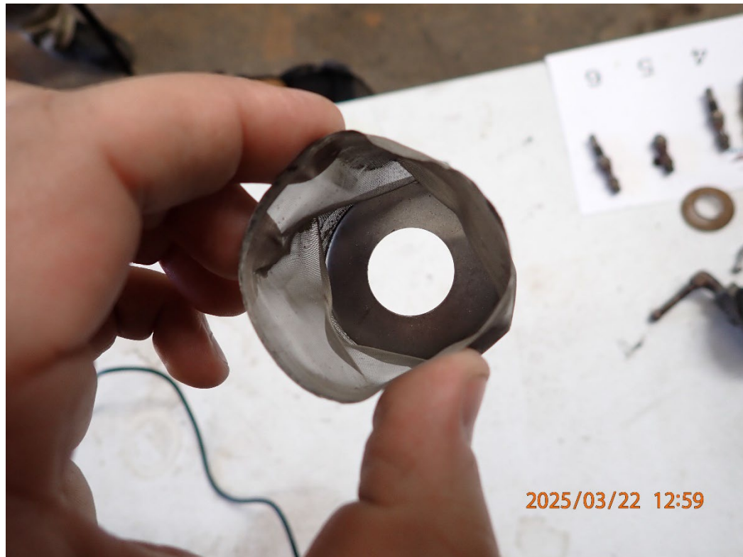
Photo 12: View of the gascolator screen.
