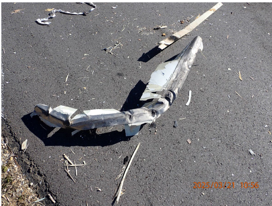
Photo 6: View of a piece of right wing leading edge found in the debris path.
