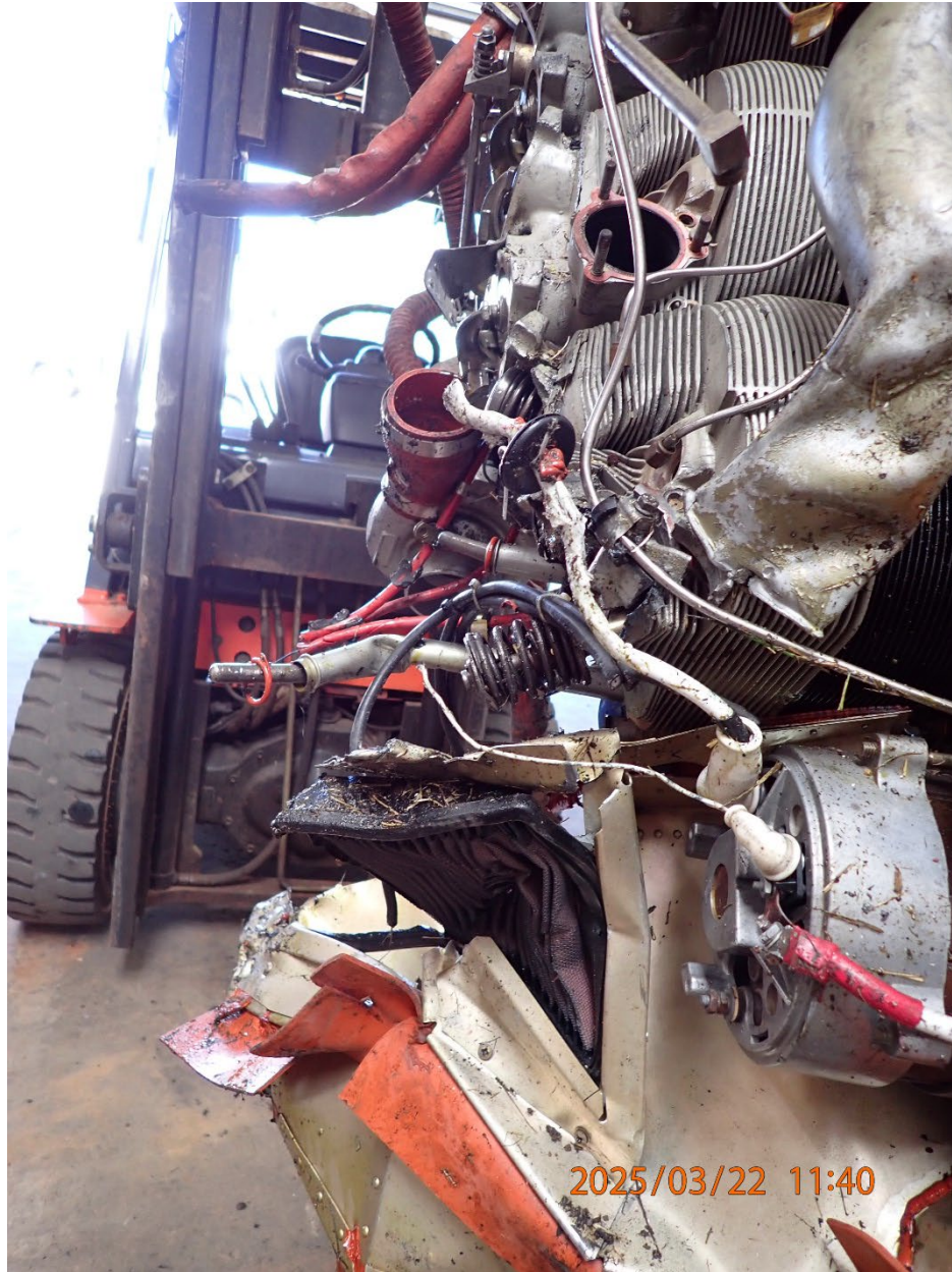
Photo 16: View of damage to the No. 5 cylinder.
