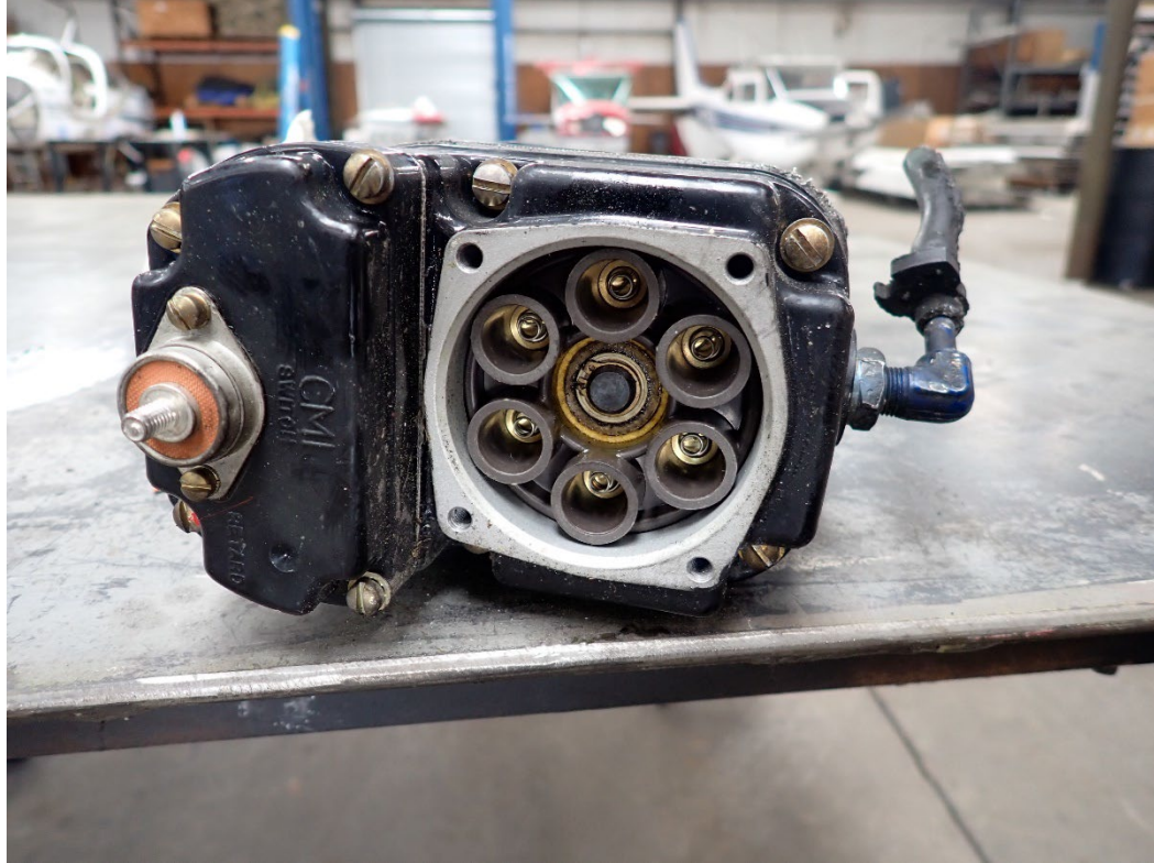
Photo 18: View of the standard magneto. (Continental Photo)
