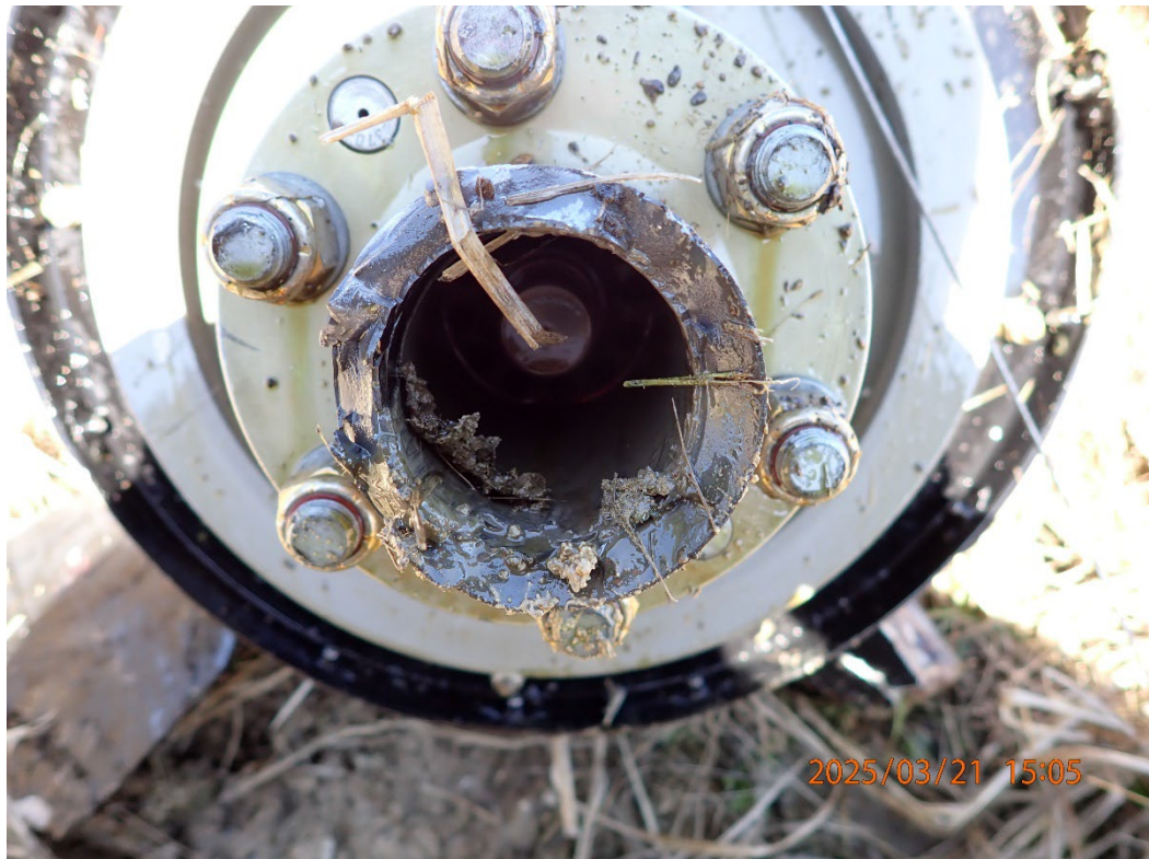
Photo 27: View of the sheared crankshaft flange attached to the propeller.
