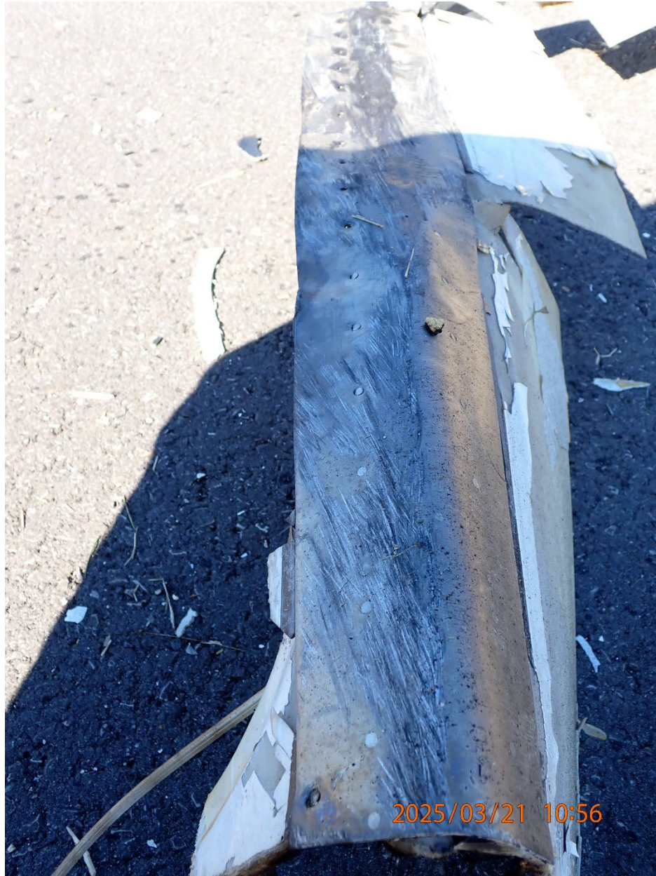
Photo 7: View of lateral scratching on the right wing leading edge piece.
