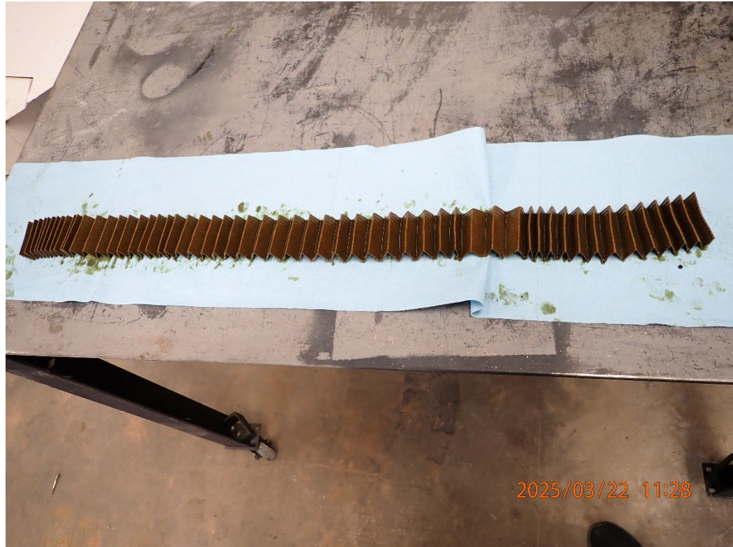
Photo 25: View of the oil filter pleats.
