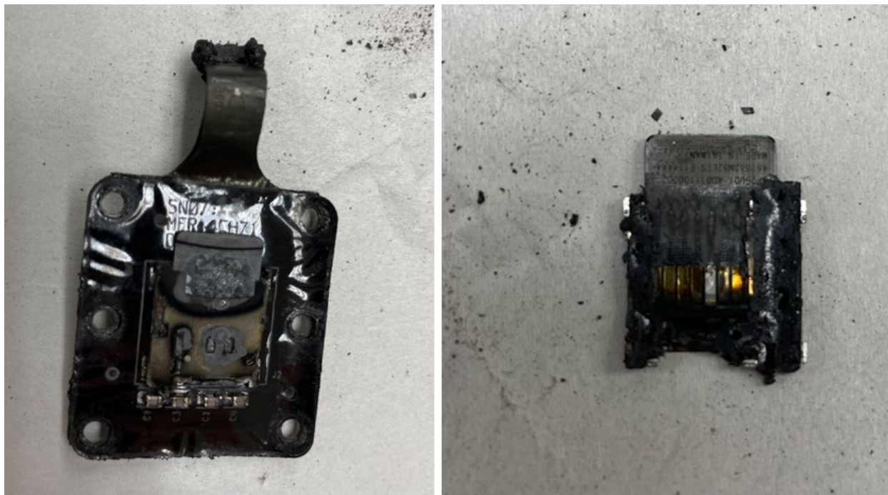
Figure 4. Severely fire damaged Avidyne DFC-90 internal microSD card.
