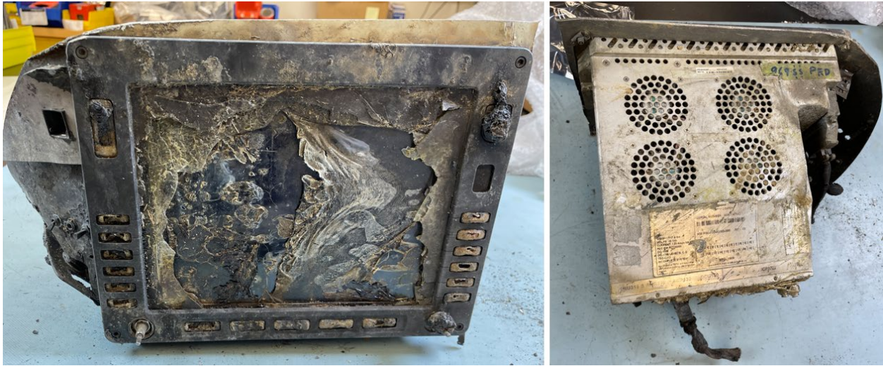
Figure 1. Front and top views of Avidyne IFD5000 - PFD as received by the NTSB Vehicle Recorder Laboratory.
