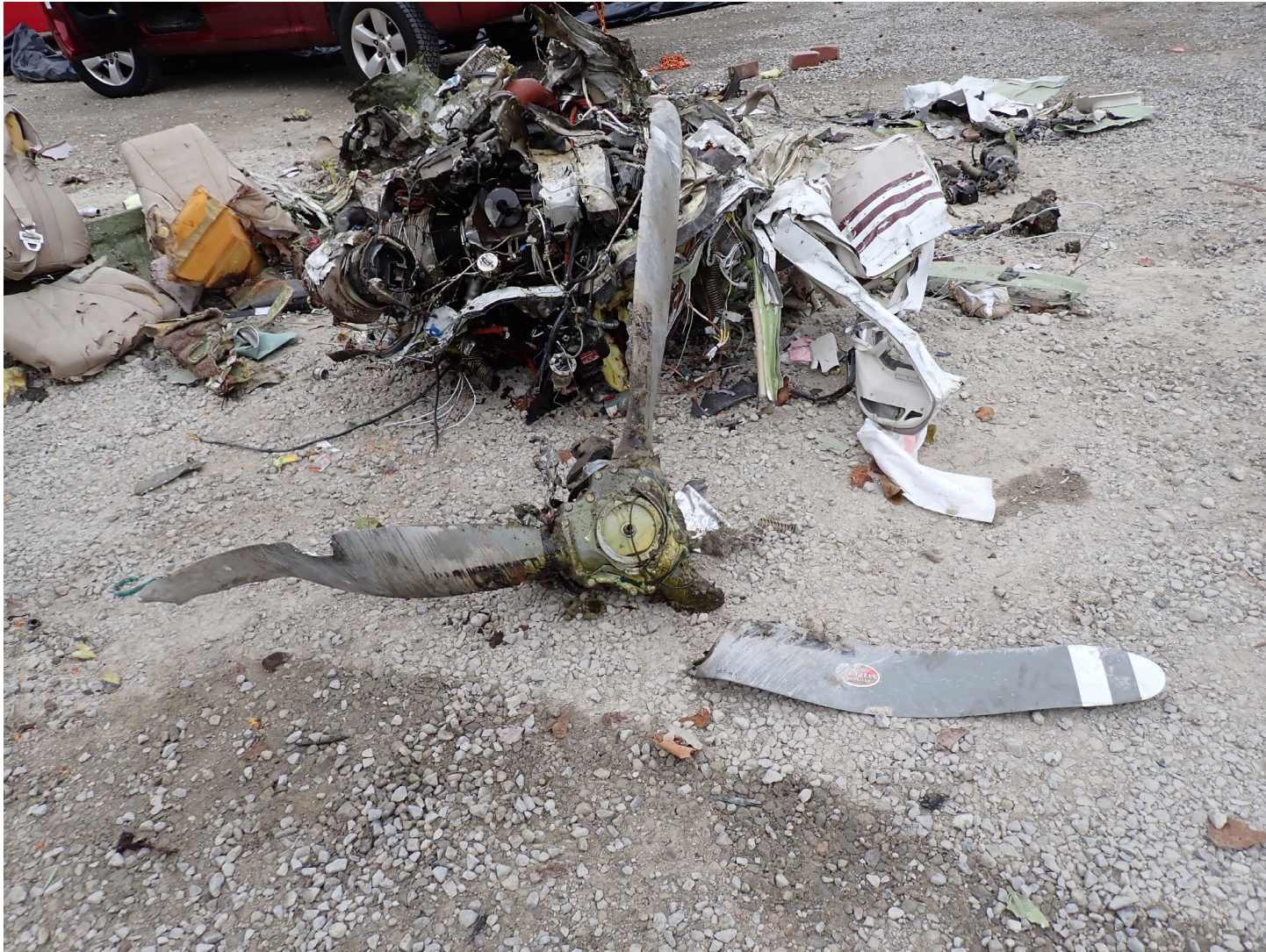
Photograph 4 - Propeller damage after recovery. (NTSB)
