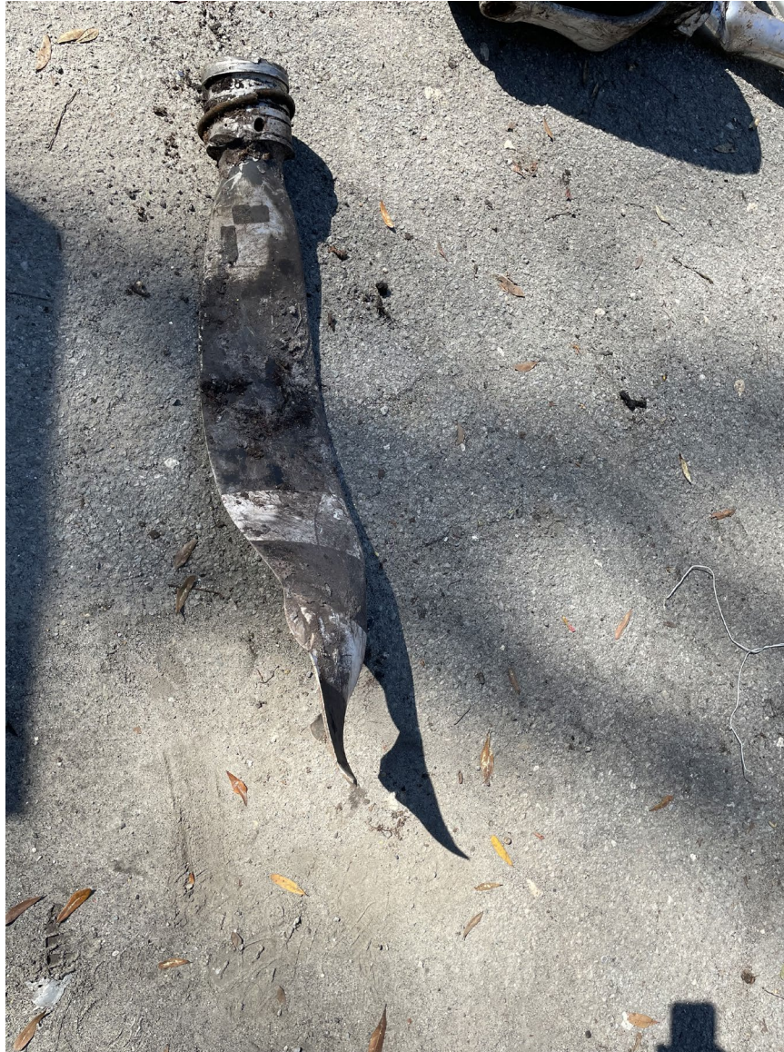
Photograph 6 - View of damaged propeller blade. (NTSB)
