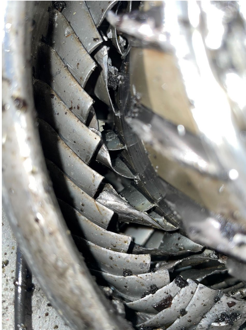
Photograph 9 - Closeup view of damaged compressor blades and stator airfoils. (NTSB)
