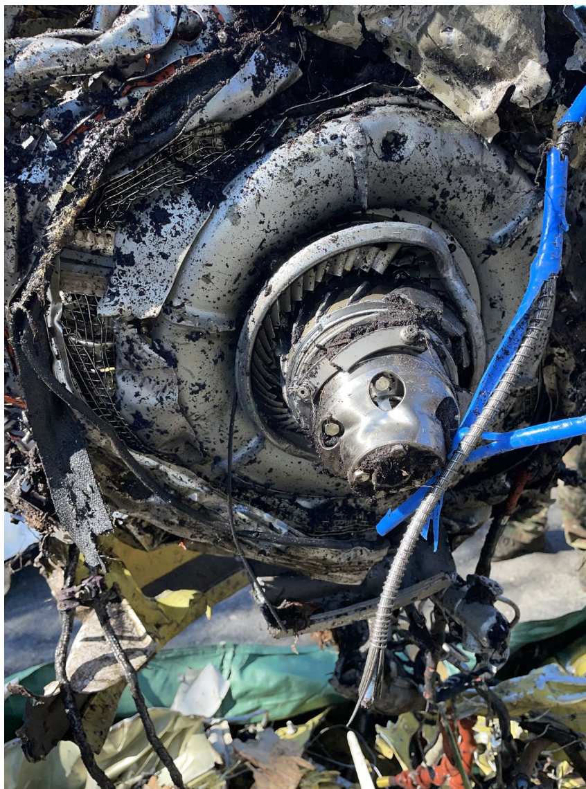
Photograph 8 - View of impact damaged engine compressor section. (NTSB)
