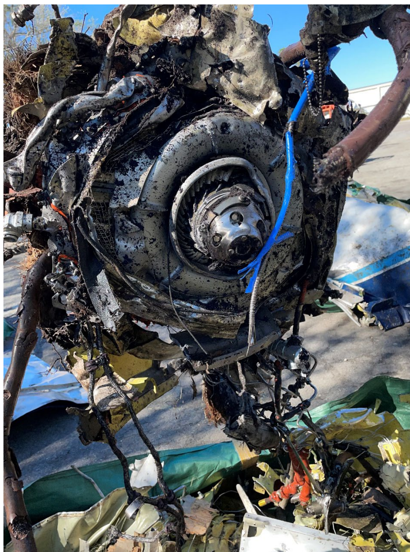
Photograph 7 - View of impact damaged engine after recovery. (NTSB)
