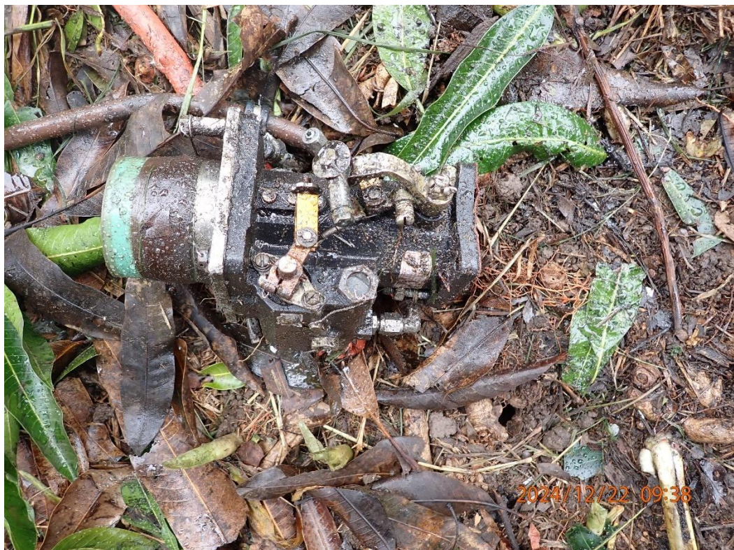
Photo 35: View of the fuel injector assembly.
