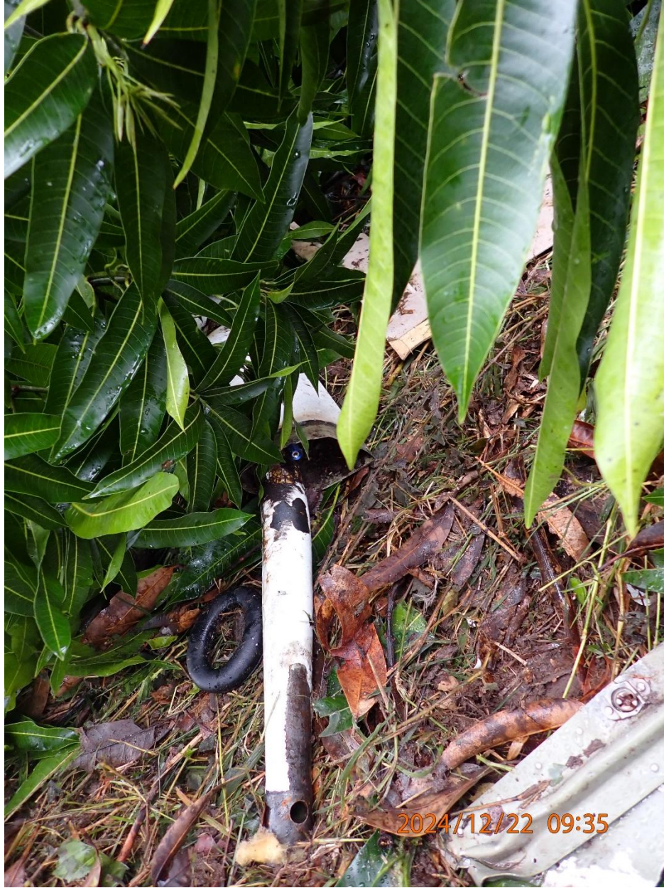
Photo 21: View of the impact separated right main landing gear.
