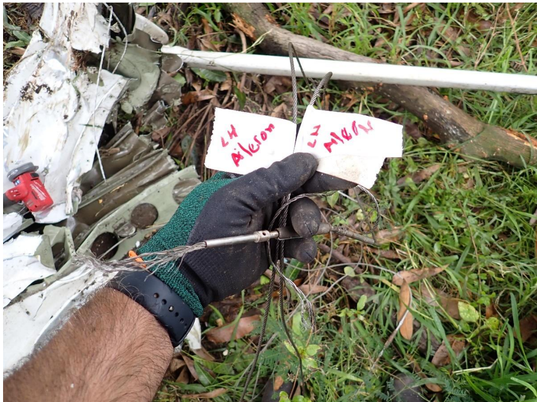
Photo 16: View of the left aileron control cables.
