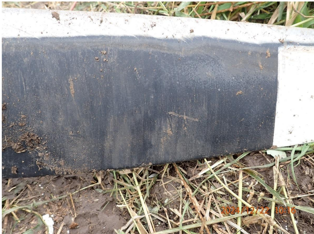
Photo 46: View of chordwise scratching and leading edge polishing/scratching.
