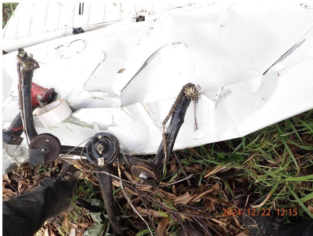
Photo 22: View of the control yoke.
