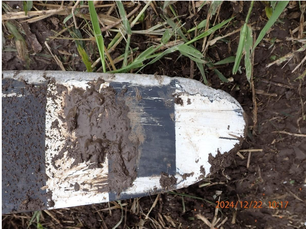
Photo 49: View of blade tip damage.
