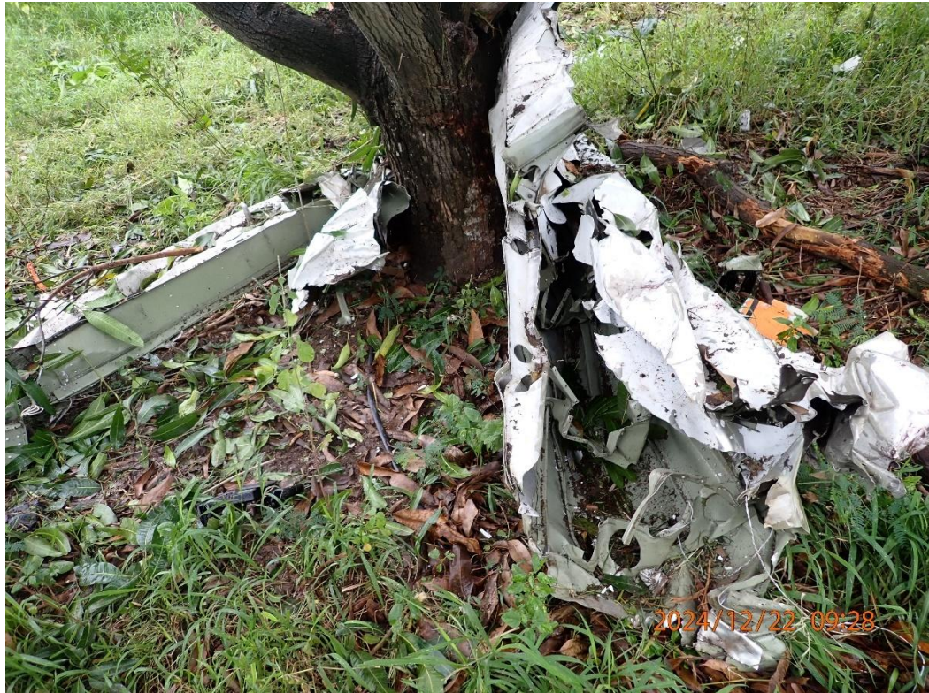
Photo 13: View of the left wing wrapped around a tree.
