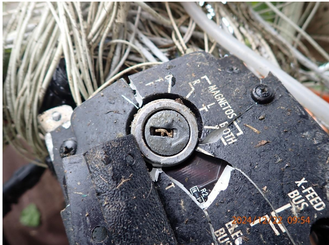
Photo 33: View of the ignition key broken in the BOTH position.
