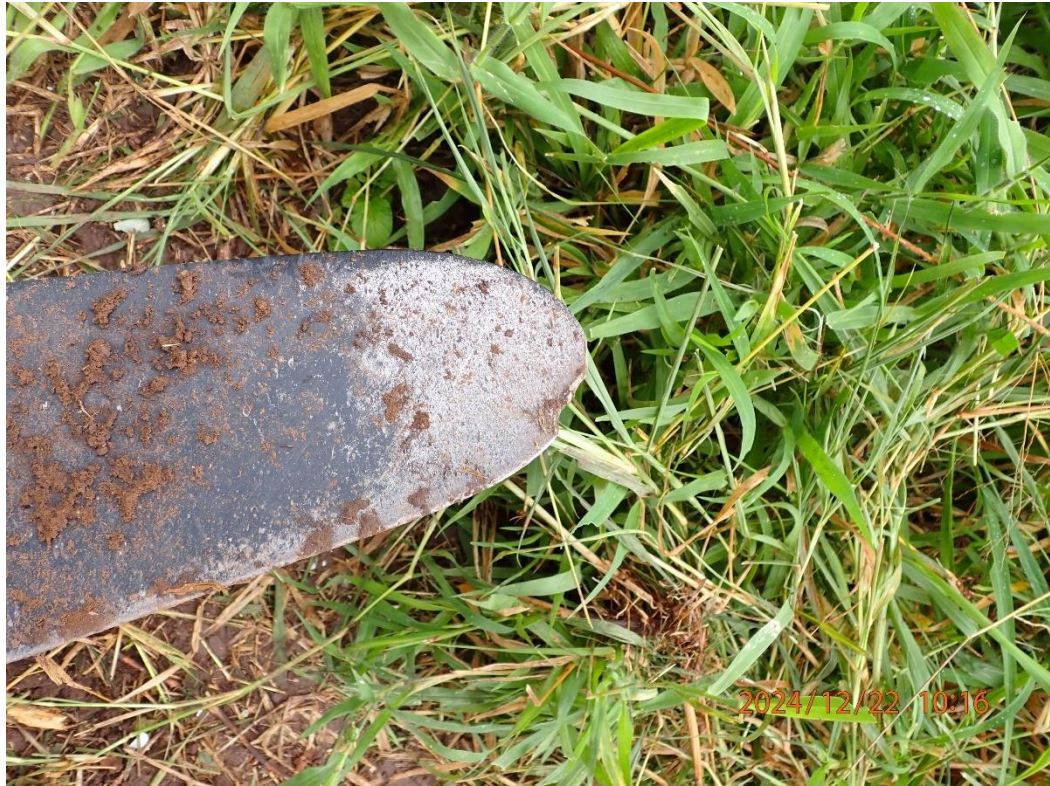
Photo 47: View of blade tip damage.
