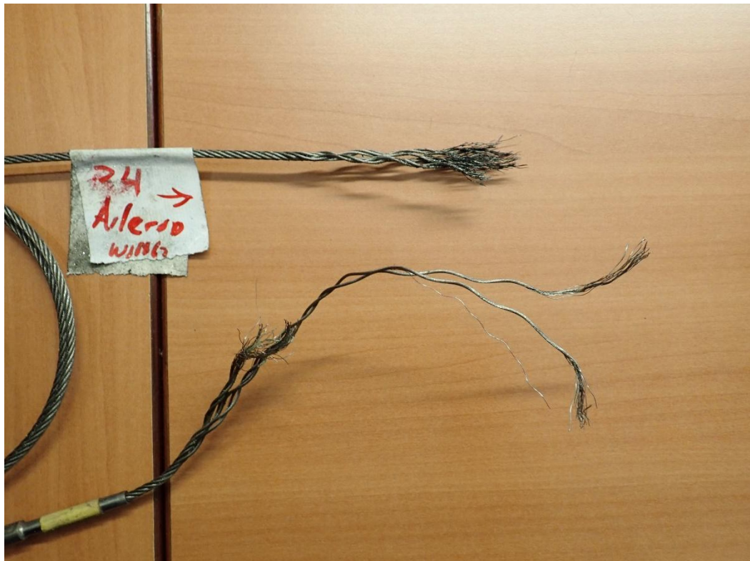
Photo 19: View of the right aileron control cable ends.
