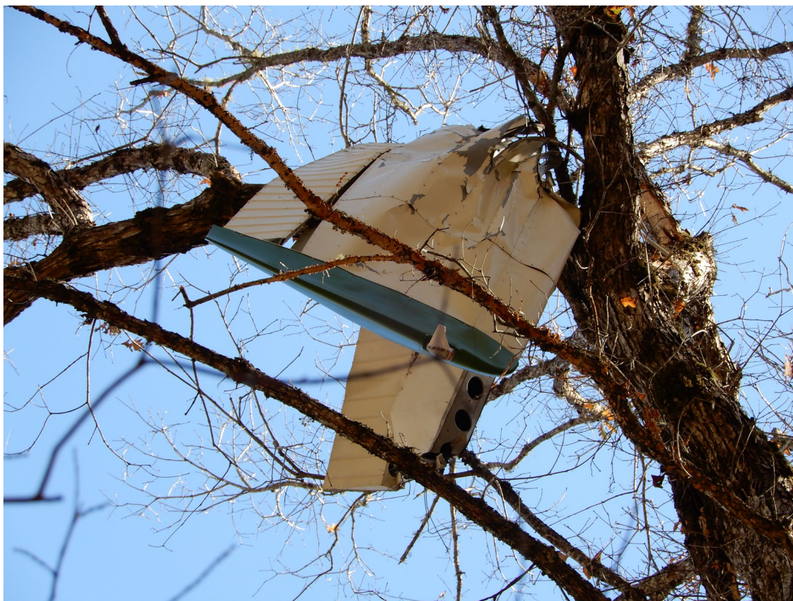
Photograph 7 - Left Wing Outboard Section (NTSB Photo)
