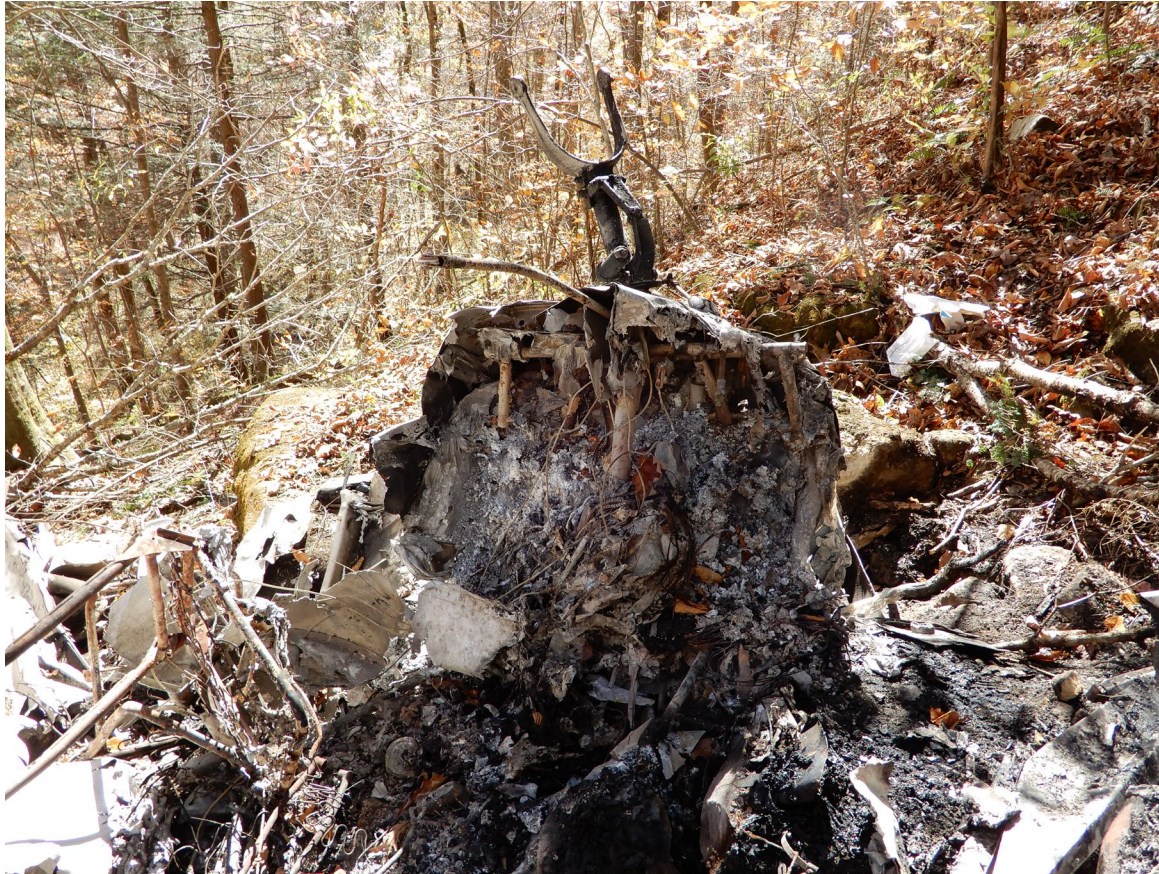
Photograph 2 - Cockpit Area and Firewall (NTSB Photo)
