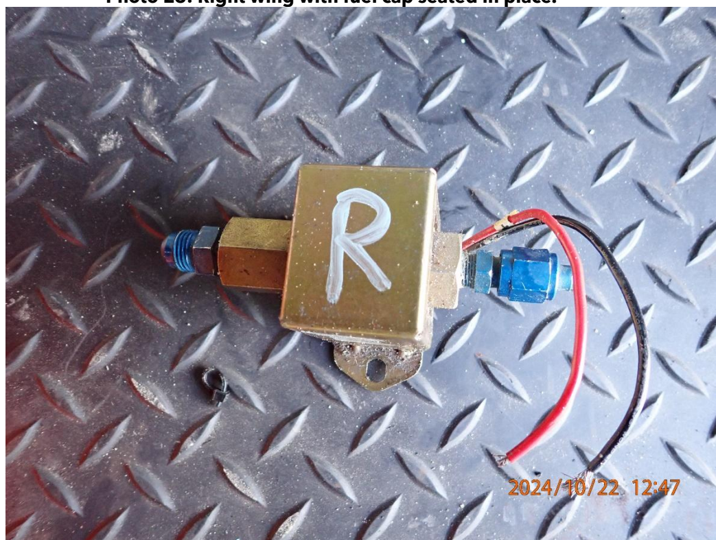
Photo 24: Right wing fuel tank pump.
