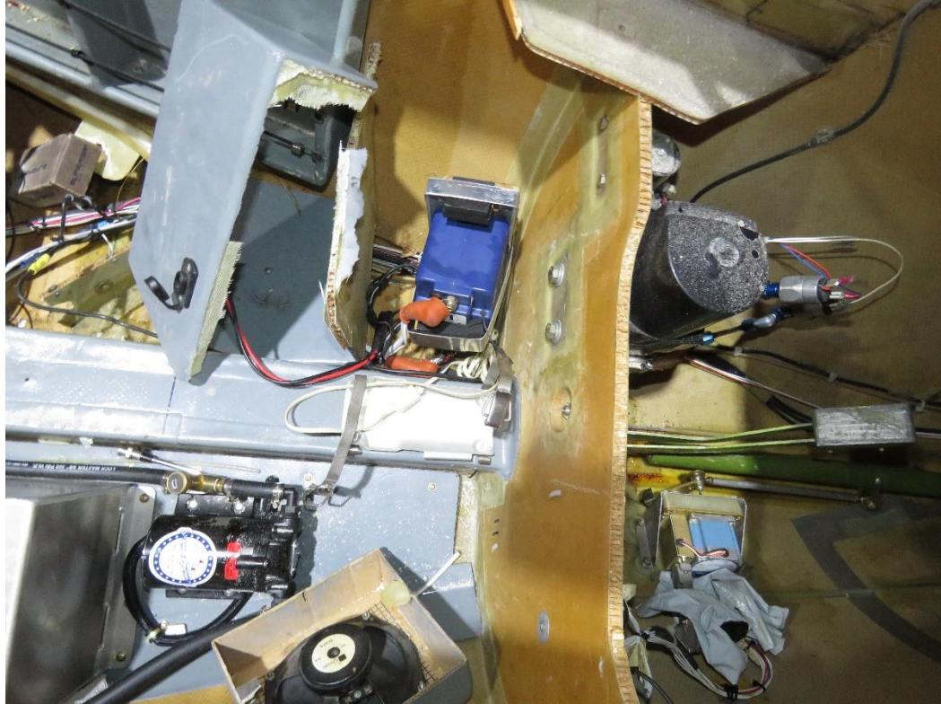
Photo 30: View of the blue main battery installed in the airplane. (Courtesy of Lycoming)
