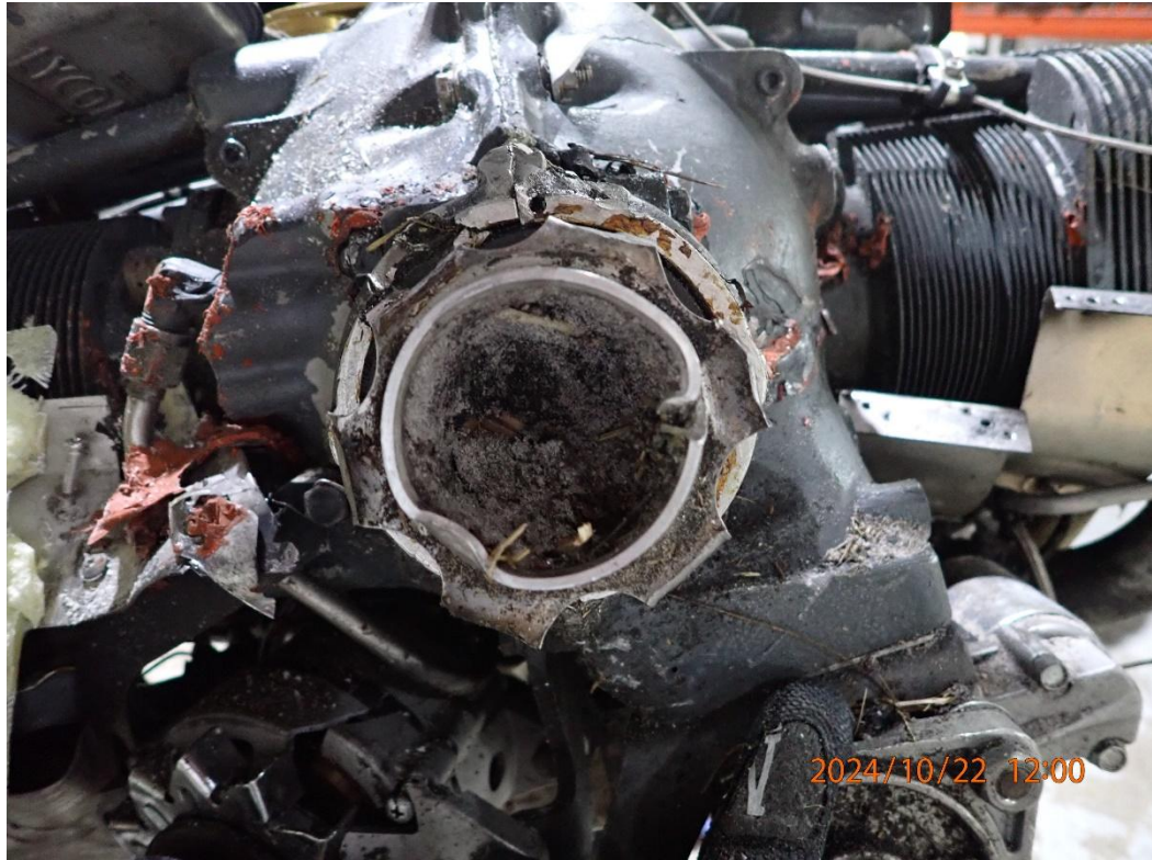
Photo 31: View of the sheared crankshaft propeller flange.
