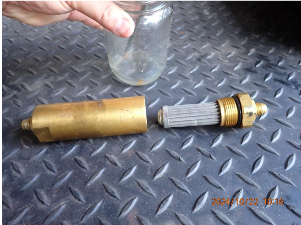
Photo 27: In line fuel filter from header tank to engine.
