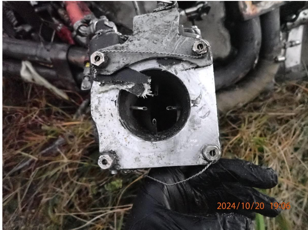
Photo 33: View of the unobstructed fuel servo venturi at the accident site.
