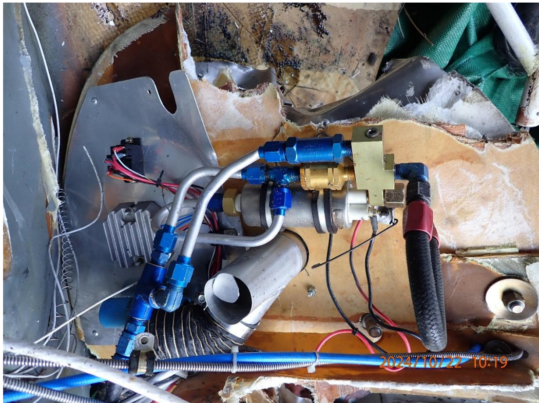
Photo 28: Header tank fuel pump assembly.
