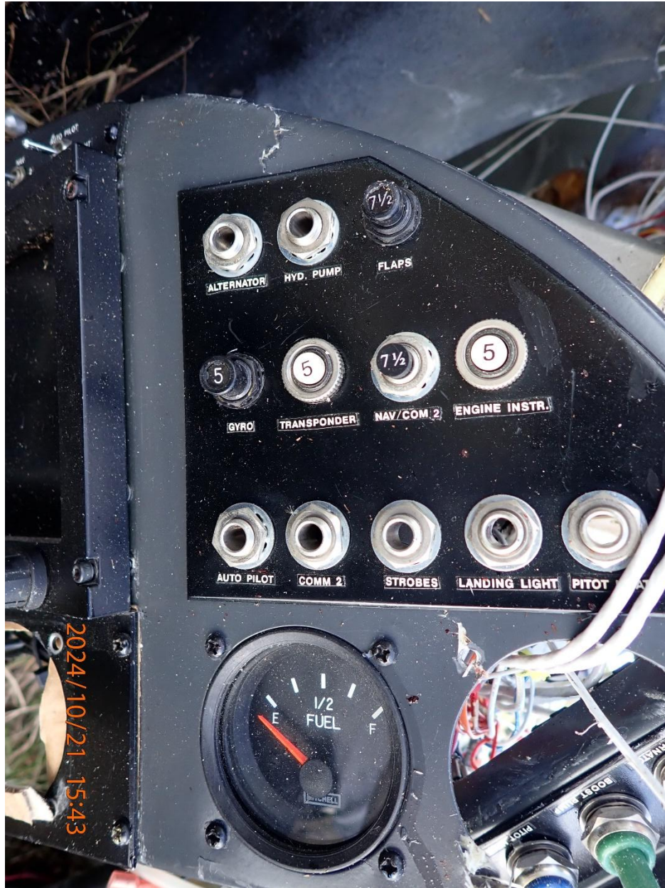
Photo 17: Circuit breaker panel
