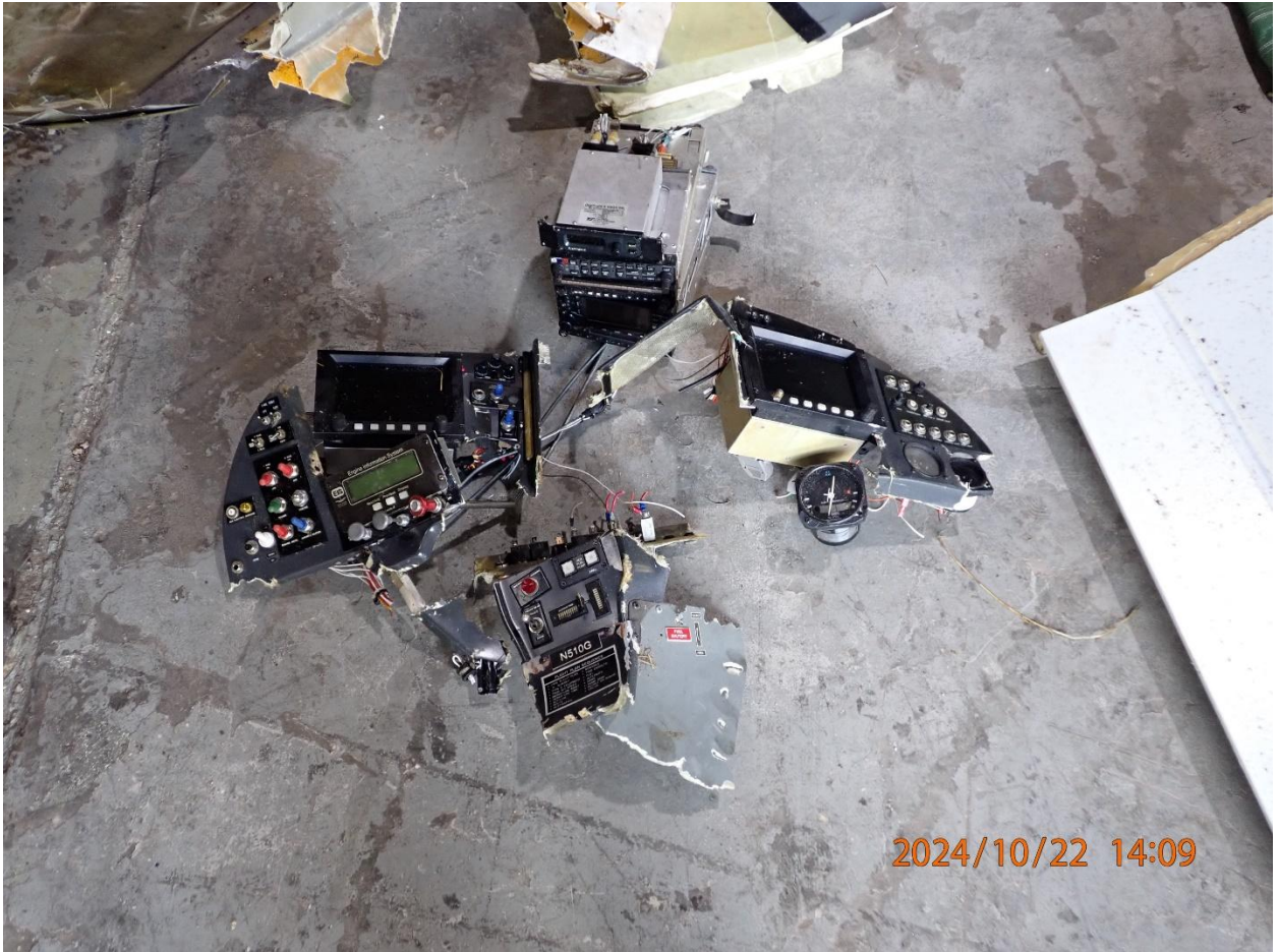
Photo 18: Layout of recovered pieces of the instrument panel.
