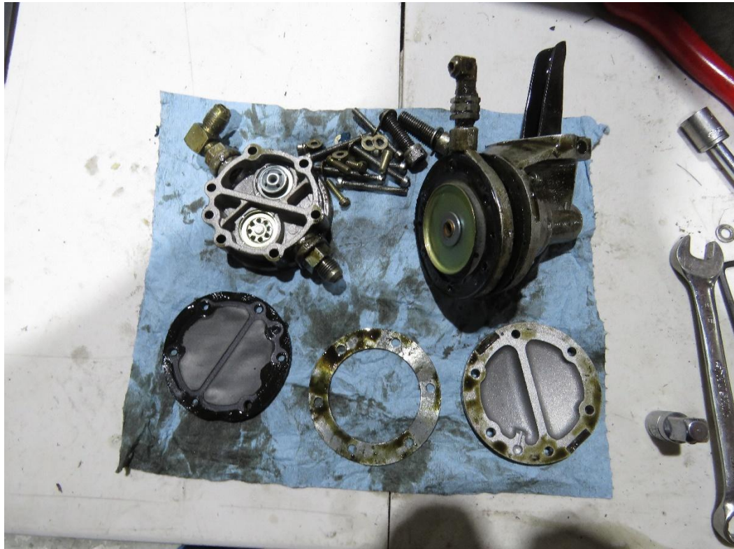
Photo 36: View of the disassembled engine driven fuel pump. (Photo courtesy of Lycoming)
