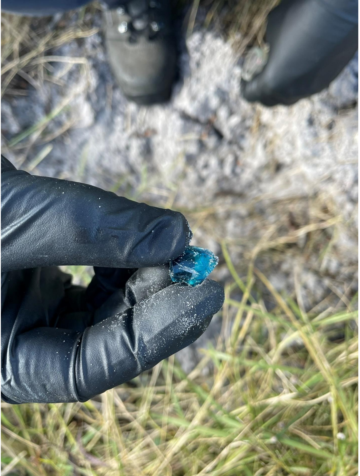
Photo 8: Lens glass found in the initial ground impact scar.
