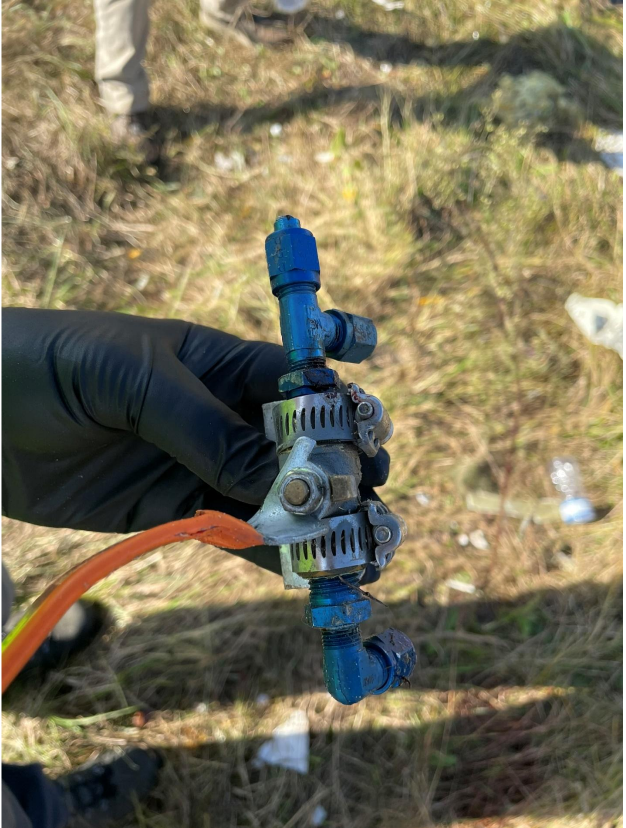
Photo 14: Landing gear dump valve.
