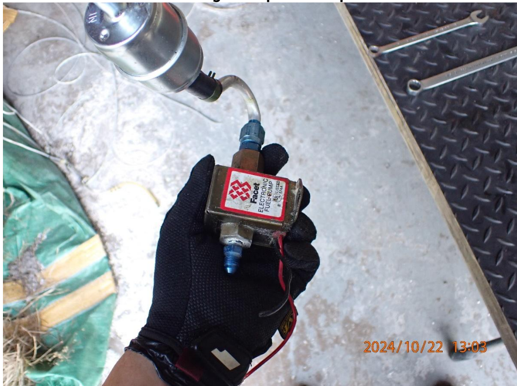
Photo 22: Left wing fuel tank in line filter and pump.
