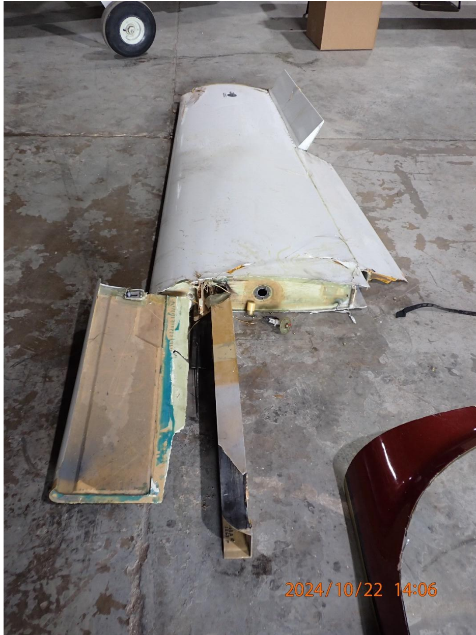
Photo 9: Identifiable portions of the right wing laid out at the recovery facility.
