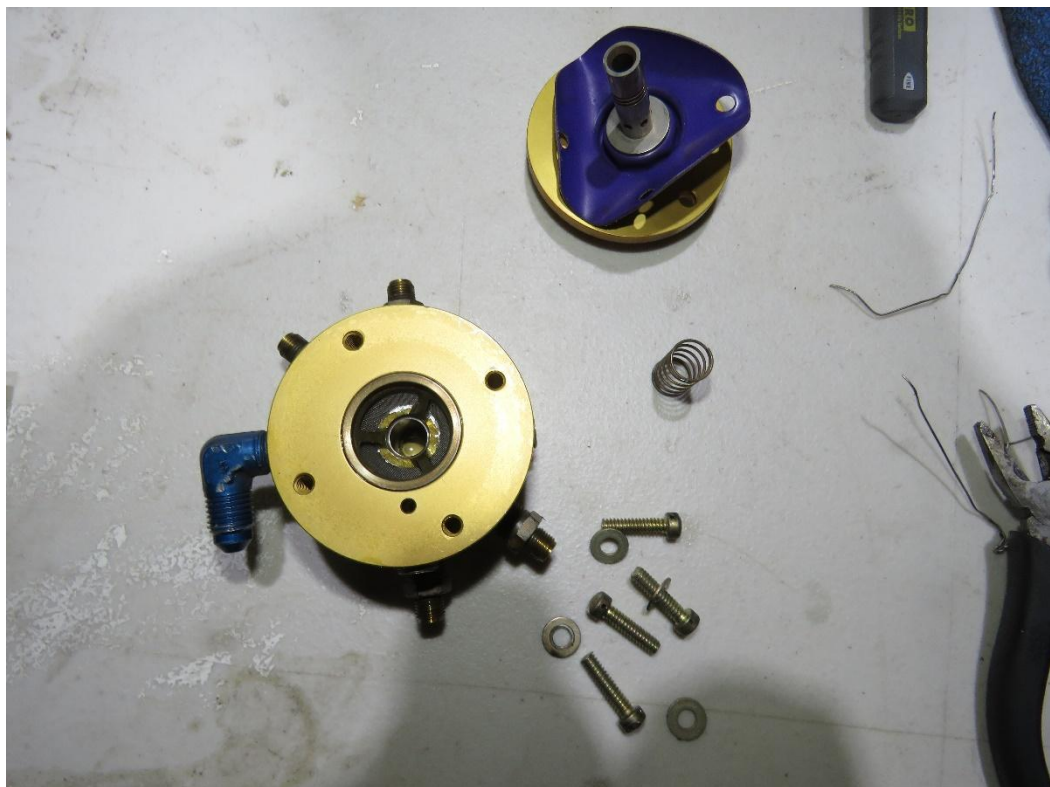
Photo 38: View of the disassembled flow divider. (Photo courtesy of Lycoming)
