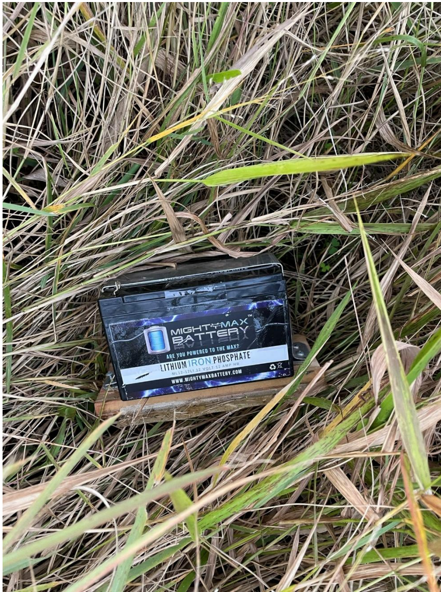
Photo 29: View of the impact separated standby battery.
