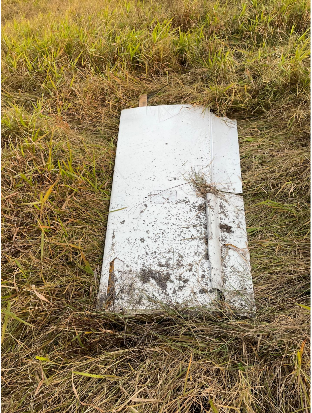
Photo 7: Outboard portion of the right wing in situ at the accident site.
