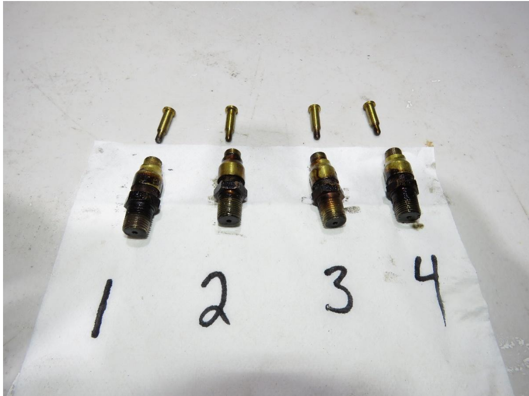
Photo 39: View of the fuel injection nozzles. (Photo courtesy of Lycoming)
