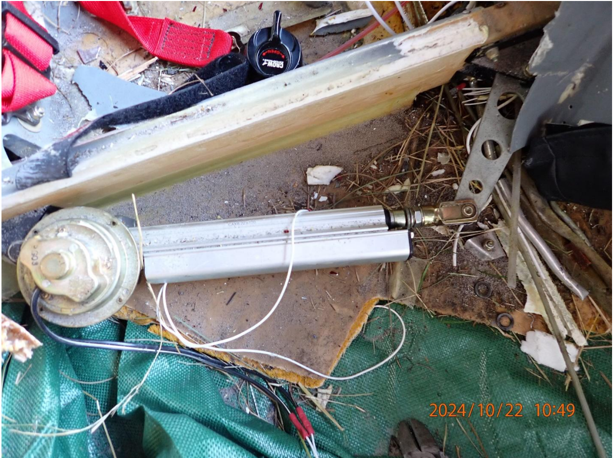
Photo 11: View of the fully retracted flap motor at the recovery facility.
