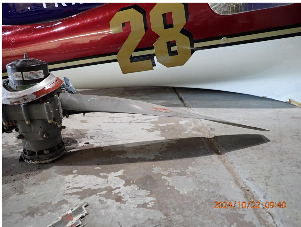
Photo 43: View of bend in blade A.
