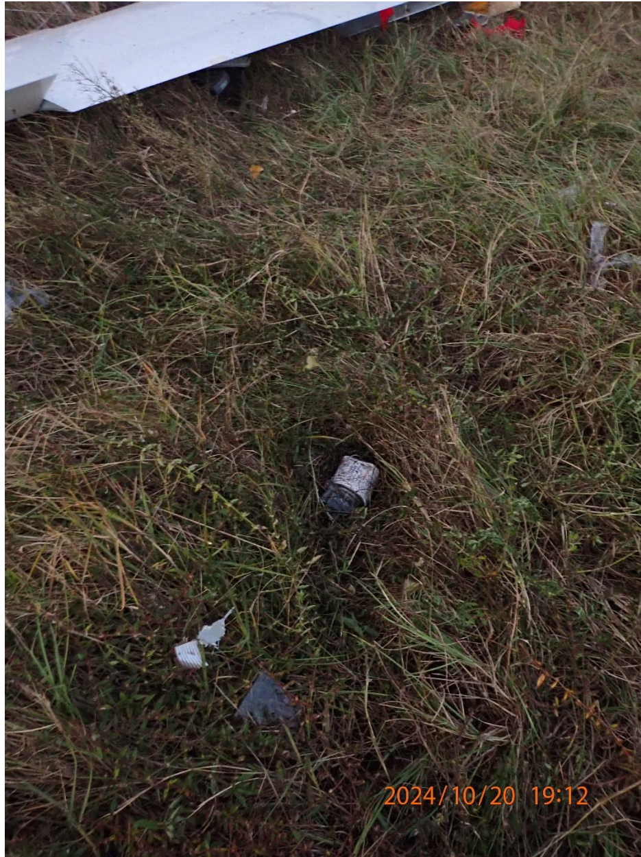
Photo 41: View of the impact separated oil filter at the accident site.
